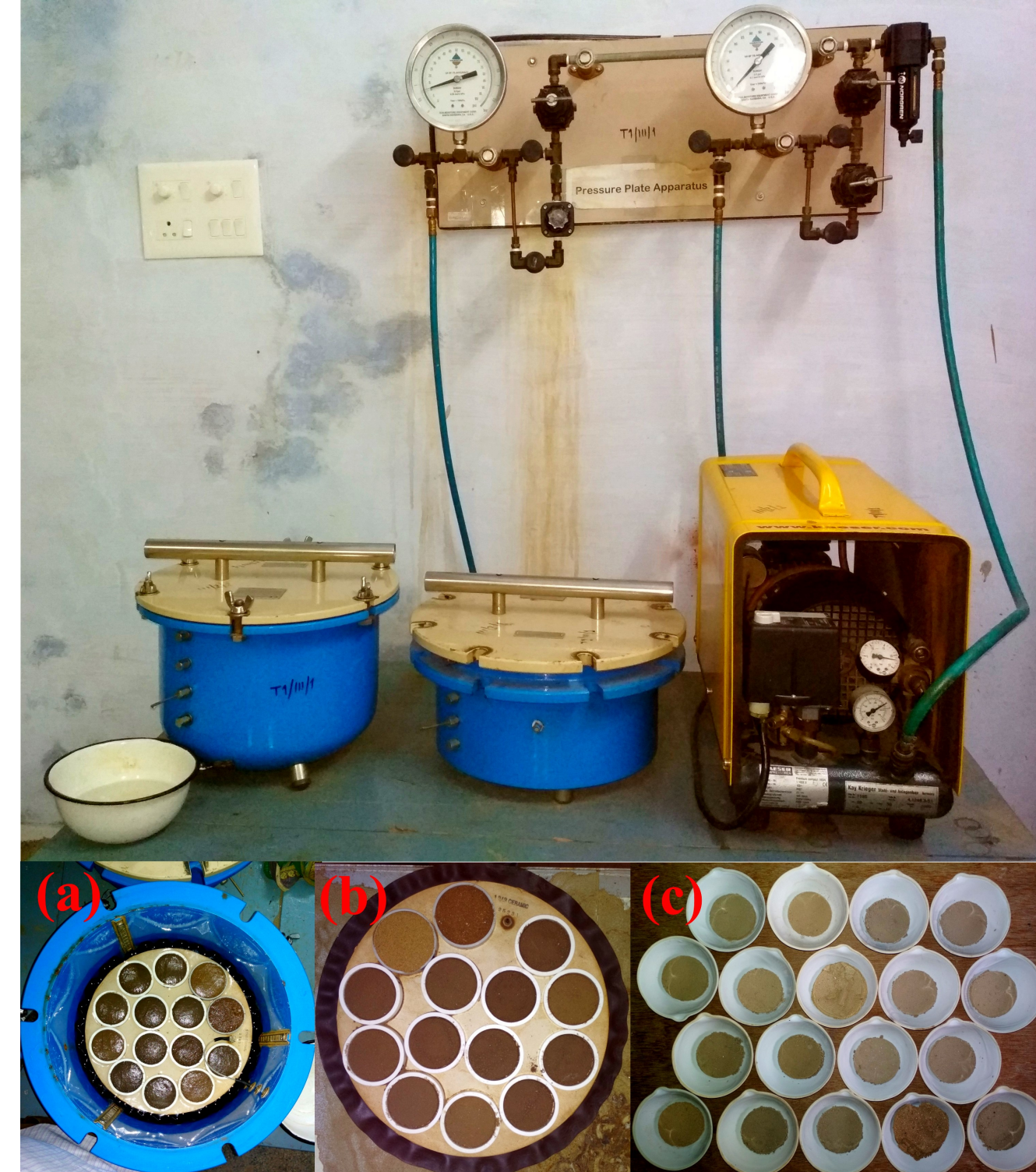
Fig.3: Pressure plate apparatus with soil samples in the states of (a) saturated, (b) equilibrium pressure and (c) oven dry
