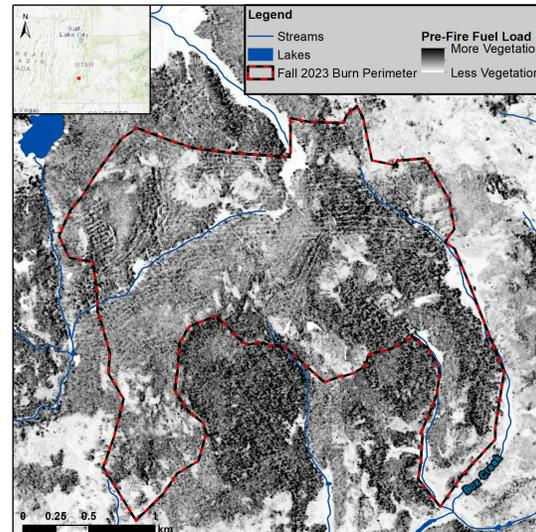
Single HV image (07/27/2023) showing pre-fire fuel availability. Two flight lines (fishla\_01601, fishla\_19601) are merged using a weighed incidence angle method. Striped features within the burn perimeter show "slash lines" where timbers are placed to aid fire managers with ignition.
