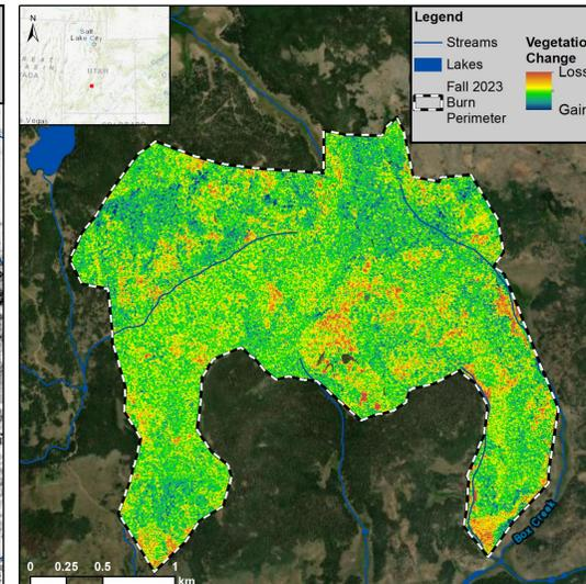
HV log ratio pre- (07/27/2023) and post- (10/17/2023) burn within the burn perimeter. High values (orange/red) indicate a loss of HV and volume scattering. Low values (green/blue) show a gain of HV between the images.
