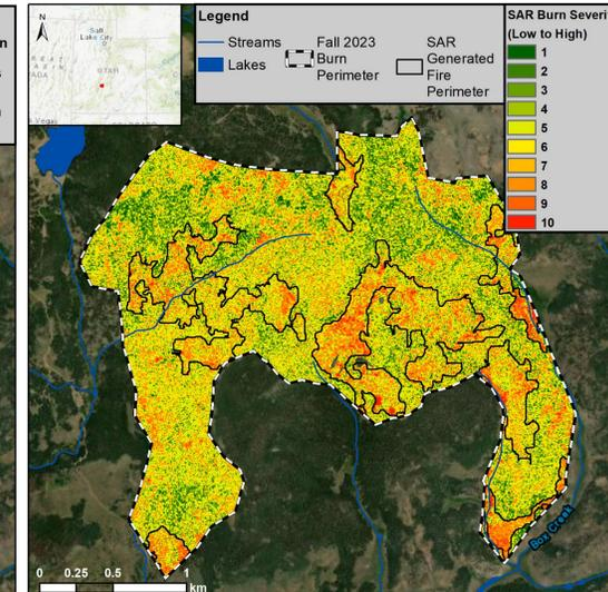
SAR-based burn severity map with 10 classes is generated from the HV log ratio image after applying k-means clustering. The small fire perimeters are also based on the HV log ratio image, after applying superpixel segmentation. The same fire perimeter method is applied to the
