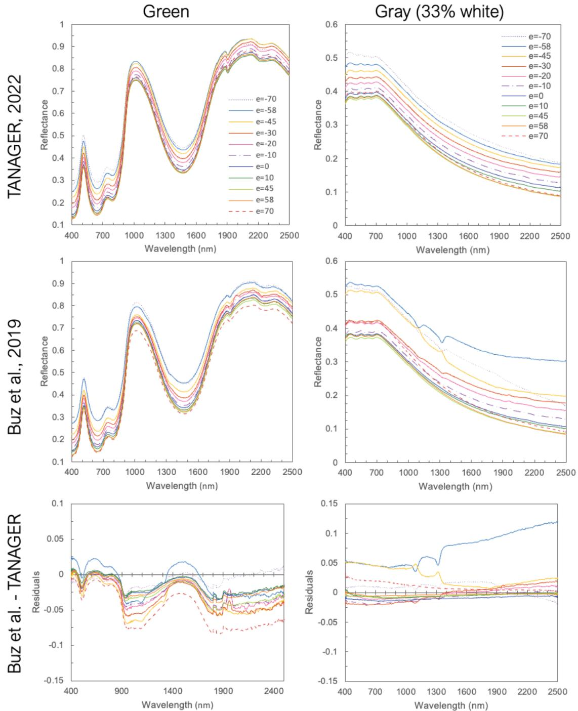
**Figure S9:** Spectra of the green and dark gray (33% white) Mastcam-Z caltarget witness samples at multiple viewing geometries from TANAGER (top) compared to Buz et al. (2019) (middle), with residuals (bottom). All measurements were acquired at  $i = 30^\circ$  and  $az = 0^\circ$ .
