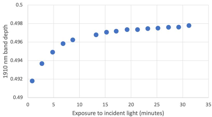
**Figure S4:** Changes to hydration band depths due to adsorbed water on anhydrite grains during continuous exposure to TANAGER's light source. Above: 1420 nm band depth beneath a continuum with shoulders at 1330 nm and 1500 nm; Below: 1910 nm band depth beneath a continuum with shoulders at 1820 nm and 2050 nm.
