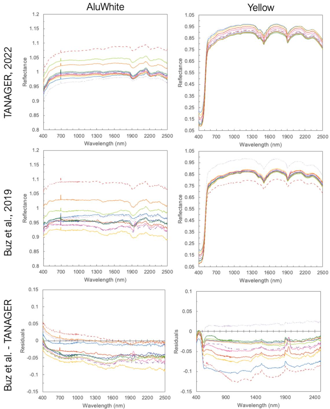
**Figure S8:** Spectra of the AluWhite and yellow Mastcam-Z caltarget witness samples at multiple viewing geometries from TANAGER (top) compared to Buz et al. (2019) (middle), with residuals (bottom). All measurements were acquired at  $i = 30^\circ$  and  $az = 0^\circ$ .
