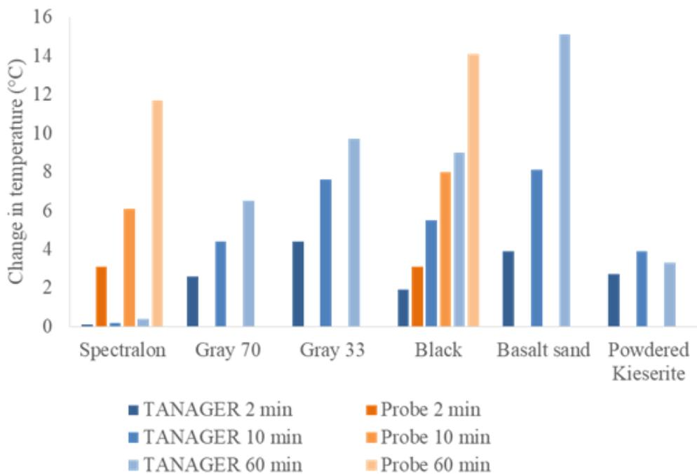
**Figure S2.** Changes in temperature under TANAGER's incident light source for a range of solid and particulate targets. Changes in temperature under a Malvern Panalytical Contact Probe for the Spectralon® and Black color standard are shown for comparison.
