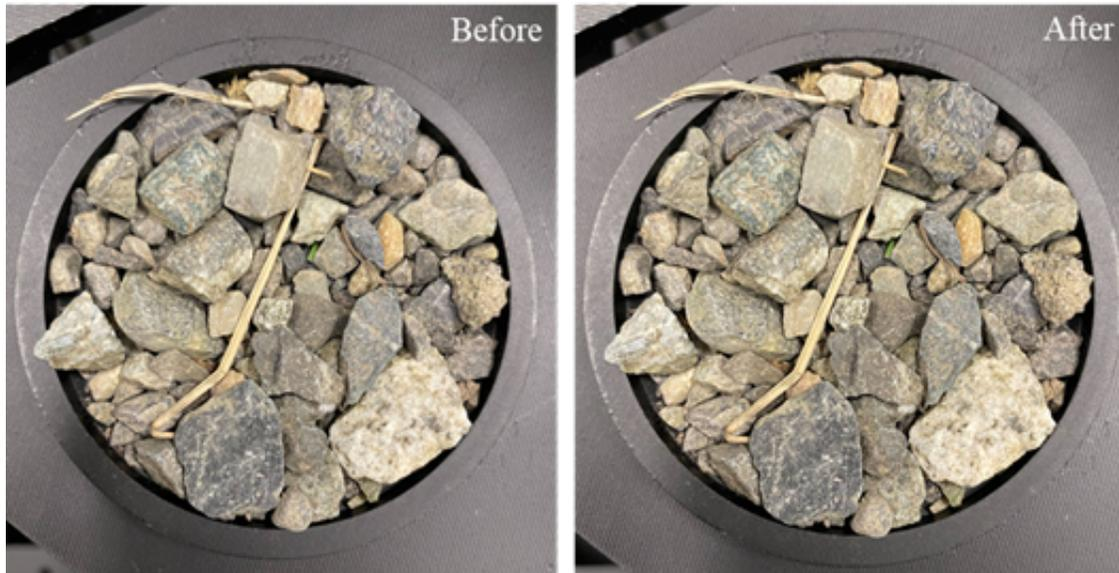
**Figure S6:** A mixture of loose gravel and grass in a TANAGER sample cup before and after being subjected to a full 360° rotation of the sample tray in 60° increments; and 360° of azimuth rotation (0° to 180° and 180° back to 0°).
