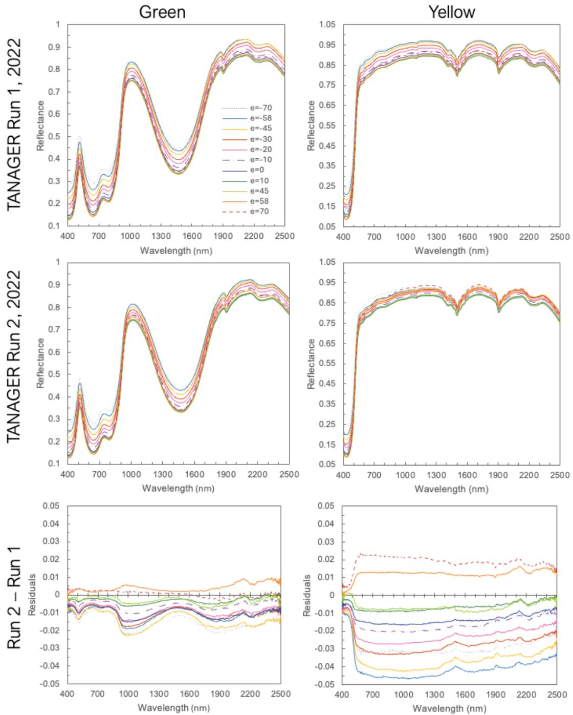
**Figure S14:** Spectra of the green and yellow Mastcam-Z caltarget witness samples from two TANAGER data collection runs (top and middle) with residuals (bottom). All measurements were acquired at  $i = 30^\circ$  and  $az = 0^\circ$ .
