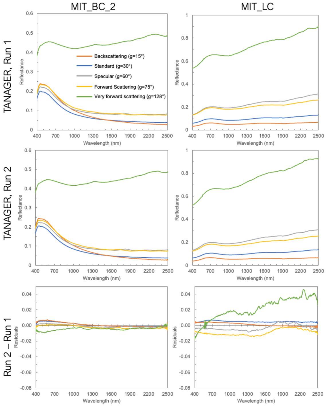
**Figure S15:** Spectra of heterogenous, naturally-coated basalt samples (MIT\_LC and MIT\_BC, see Figure 25) from two TANAGER data collection runs (top and middle) with residuals (bottom). All measurements were acquired at  $i = 30^\circ$  and  $az = 0^\circ$ .
