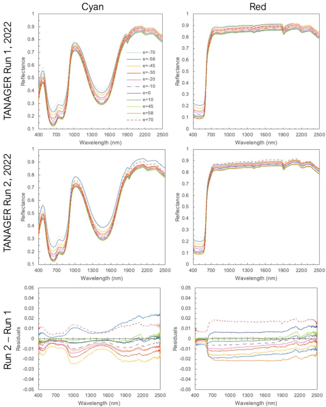
**Figure S11:** Spectra of the cyan and red Mastcam-Z caltarget witness samples from two TANAGER data collection runs (top and middle) with residuals (bottom). All measurements were acquired at  $i = 30^\circ$  and  $az = 0^\circ$ .
