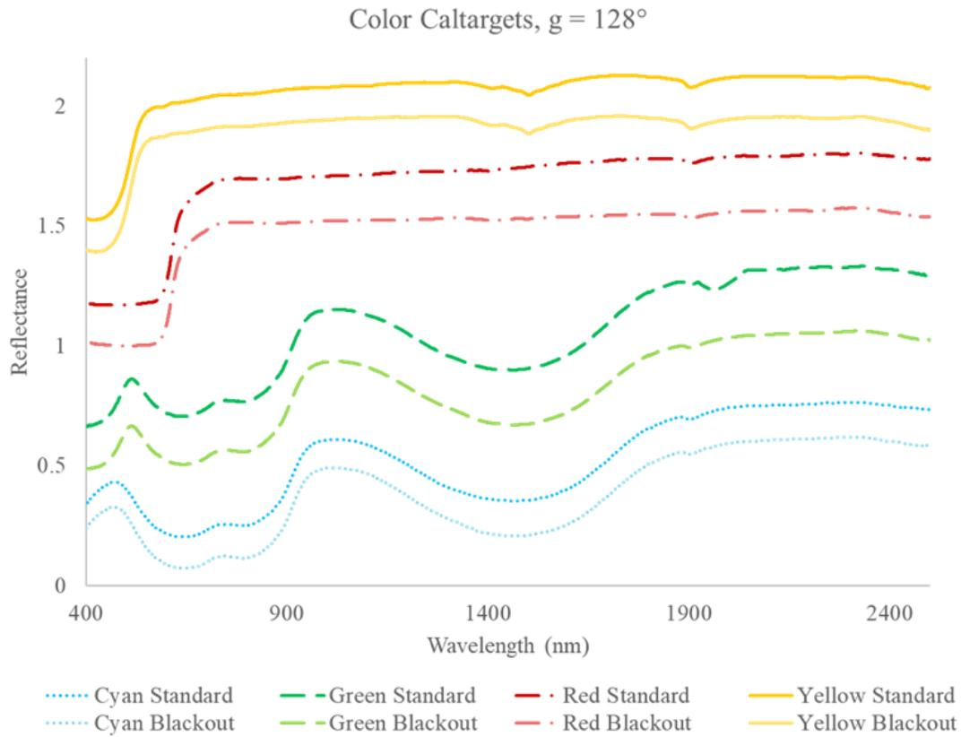
**Figure S10:** Spectra of color caltargets collected with TANAGER in a very forward-scattering geometry ( $g = 128^\circ$ ) with and without blackout curtains on the lab cabinetry (“Blackout” vs. “Standard”). The curtains reduce stray light reflected from lab surfaces and reduce overall reflectance (but do not otherwise change spectral shape). Spectra are offset for clarity (Cyan by -0.55; Green by -0.15; Red by +0.40; Yellow by +0.80).
