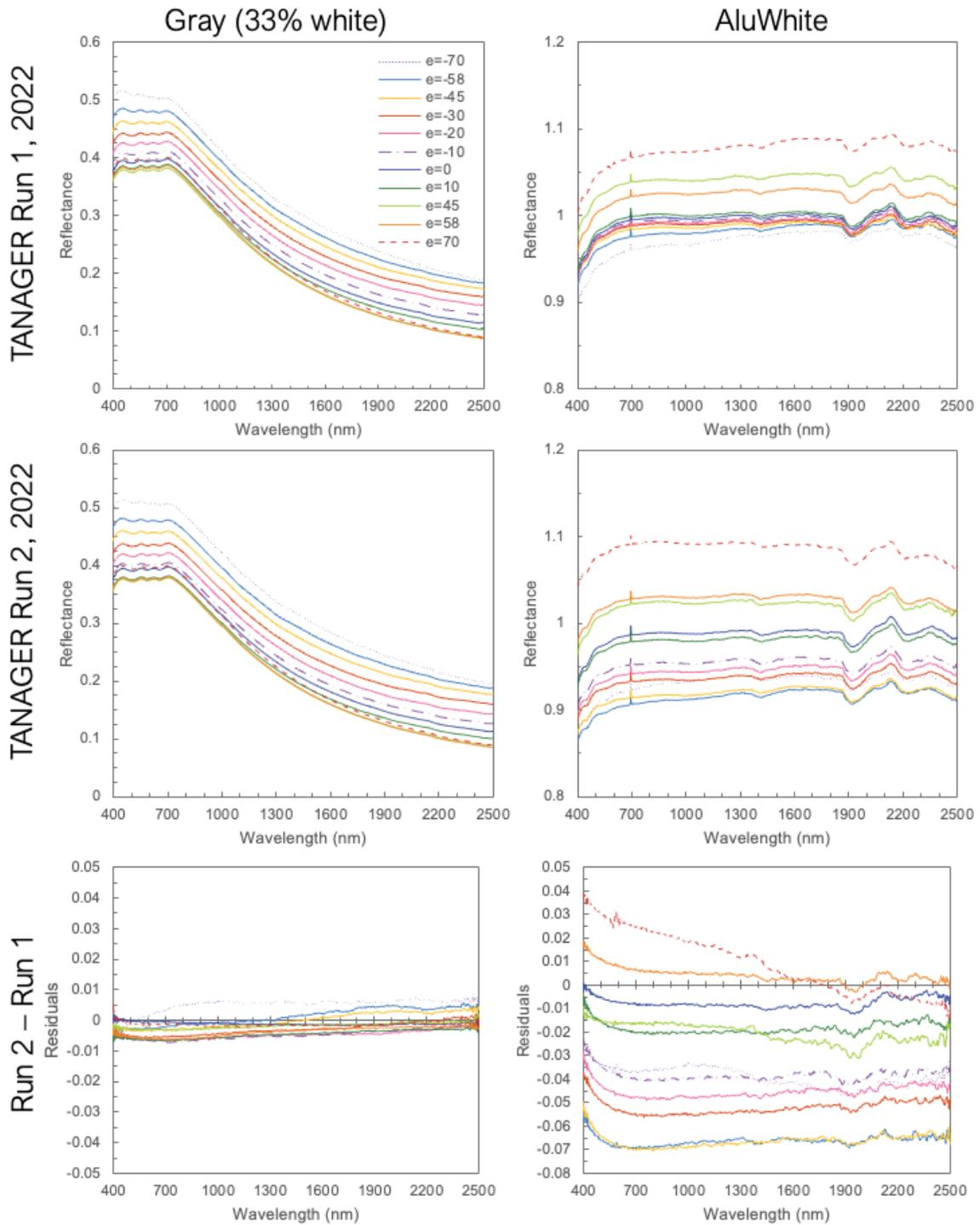
**Figure S13:** Spectra of the dark gray (33% white) and AluWhite Mastcam-Z caltarget witness samples from two TANAGER data collection runs (top and middle) with residuals (bottom). All measurements were acquired at  $i = 30^\circ$  and  $az = 0^\circ$ .
