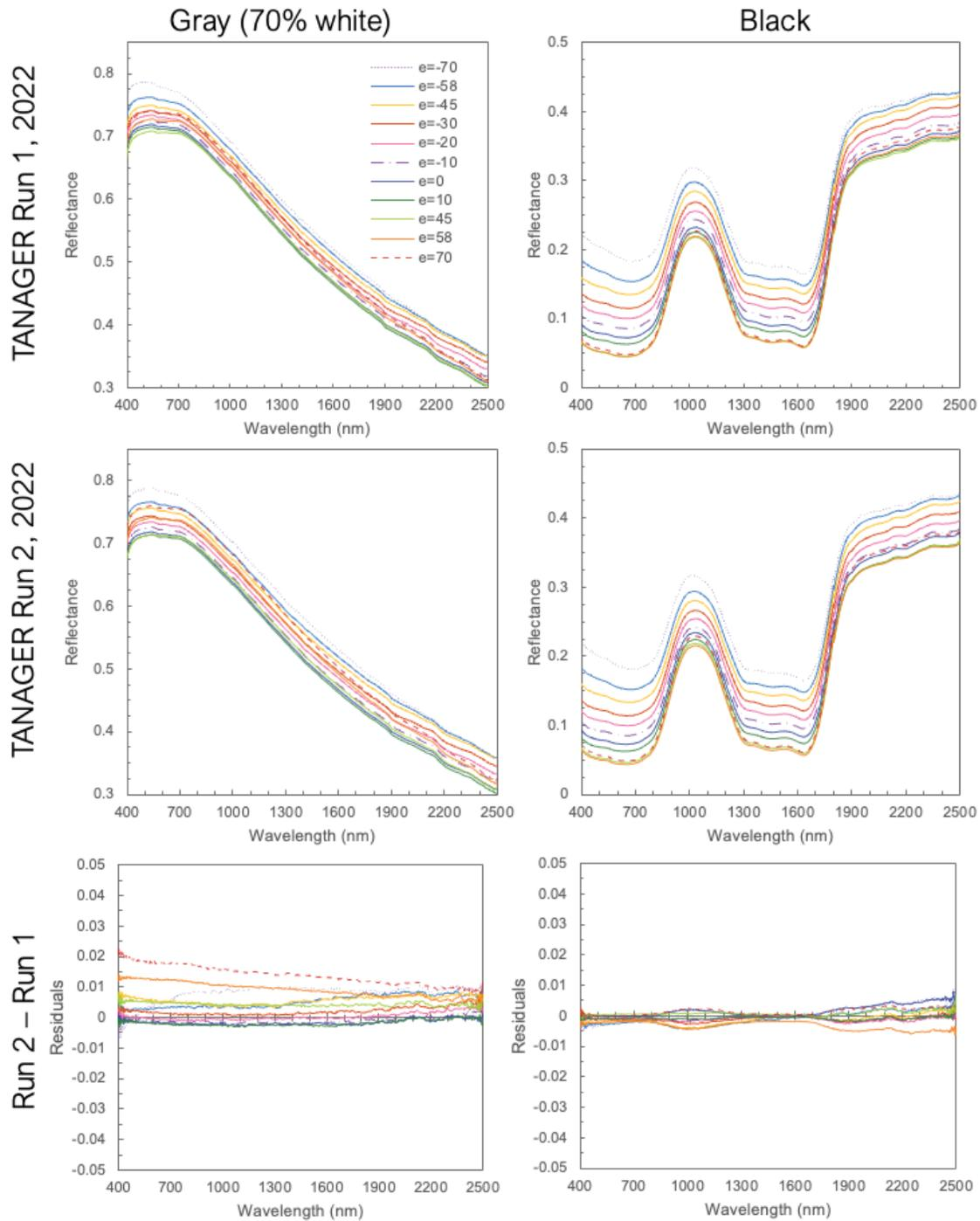
**Figure S12:** Spectra of the light gray (70% white) and black Mastcam-Z caltarget witness samples from two TANAGER data collection runs (top and middle) with residuals (bottom). All measurements were acquired at  $i = 30^\circ$  and  $az = 0^\circ$ .
