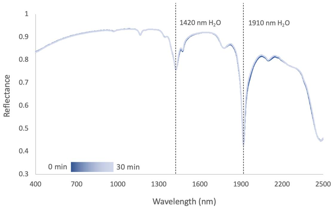
**Figure S3:** Fifteen spectra of anhydrite (CaSO<sub>4</sub>) acquired over 30 minutes of continuous exposure to TANAGER's incident light source. Prominent absorption bands due to hydration are labeled. No meaningful changes to these absorptions (or any other spectral features) were observed during heating experiments, implying that TANAGER's light source is unlikely to drive off adsorbed water from mineral grains (or otherwise dehydrate samples).
