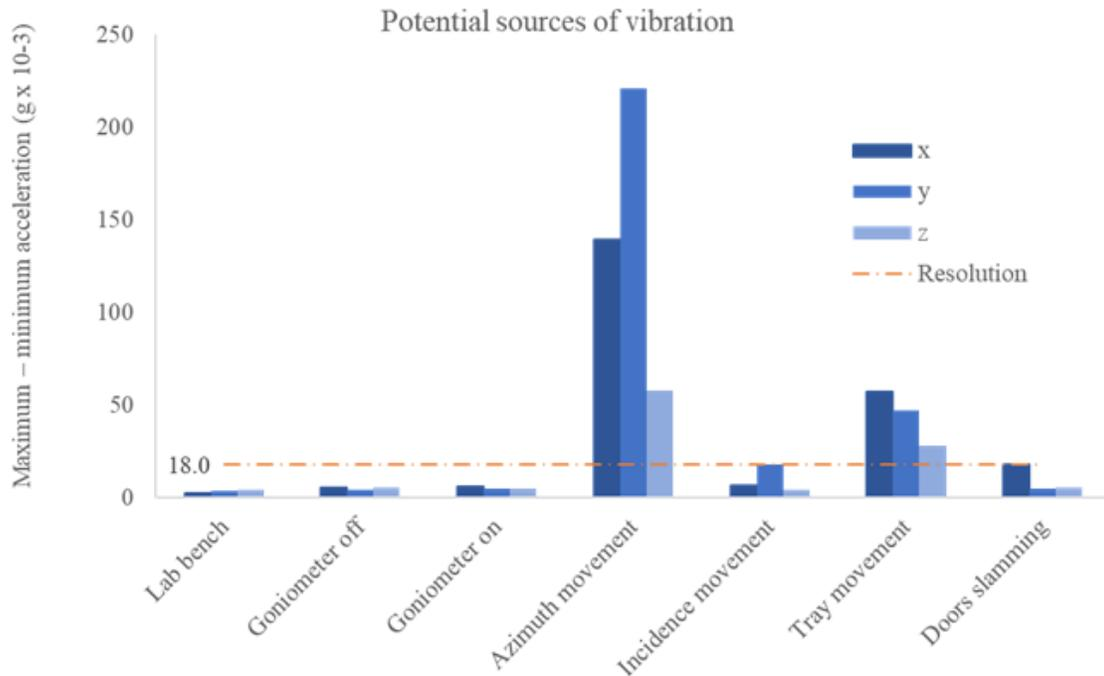
**Figure S5:** Total variation (maximum – minimum acceleration values) for x, y and z axes yielded from possible TANAGER vibration sources. The dashed horizontal line represents the resolution of the hardware and software.
