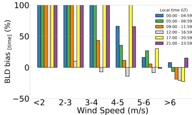
**Figure 4.** Mean boundary layer depth (BLD) bias (mean mismatch between hourly modeled and observed BLD) for different time ranges shown at local time (LT), categorized by wind speed classes, for January and February 2016.
