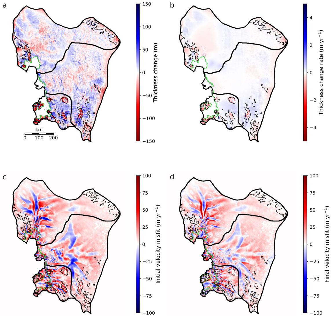
**Figure S1.** Initial state following the 50 year initialisation procedure. (a) Total thickness change from the original ice thickness. (b) Rate of thickness change after 50 years in the final relaxation iteration. (c) Initial ice velocity misfit. (d) Final ice velocity misfit. Thick black lines show the basin boundaries and ice extent while thin black lines show the sea level contour of bed depth. Grounding lines are marked by green lines.
