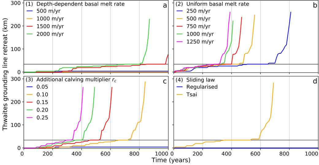
**Figure 4.** Grounding line retreat along the TG flowline for enhanced forcing experiments. Lines are truncated where the grounding line retreats beyond the end of the flowline, with the vertical scale covering the full flowline extent. Horizontal lines are drawn at 34 km.
