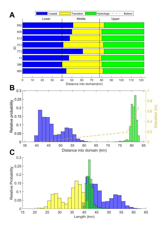
**Figure 7**. Compound flood hazard zones for the simulation subset (a), and relative probability of the compound flood hazard zone's (b) interface and (c) lengths for the entire simulation set. Each color bar represents a different compound flood hazard zone. The gold dashed line represents the idealized coastal watershed transect. The dotted lines represent the different segments within the idealized coastal watershed transect. (created using MATLAB)
