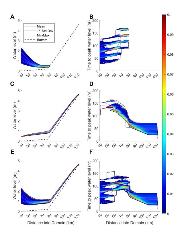
**Figure 6**. Maximum water levels (a,c,e) and time to peak water level (b,d,f) for the complete set
