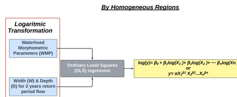
**Fig. 6.** River geometry definition
