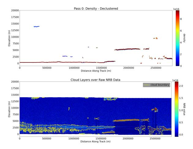
DDA-atmos uses an anisotropic Gaussian radial basis function (described by equation below) to calculate weighted photon density. Then a gradient in density represents a change in atmospheric composition.
