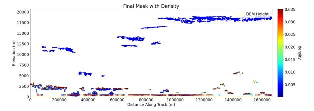
Because of the differences between satellites, simply employing the DDA built for ICESat-2 data does not yield desired results in CALIPSO data, as seen in the figure above, which misses a significant portion of the smoke layer.
