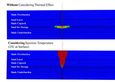
Figure 6 – Very small fracture is predicted in isothermal model, and H<sub>2</sub> is contained in storage layer after 4-cycle
