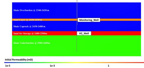
Figure 2 – Cross-section view (x-axis) of the model, showing the layering and well placement.
