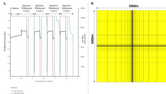
Figure 1 – (A) Injection and withdrawal control (rate and BHP) of the model, and (B) top view of saline aquifer model showing dimension and grid refinement
