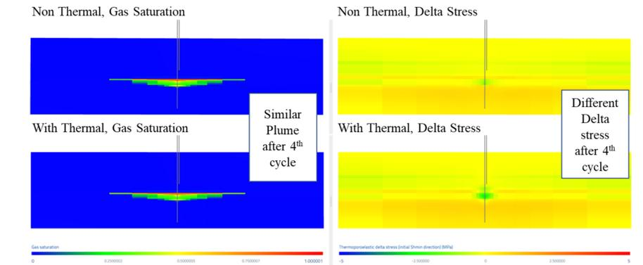
Figure 8 – Although the gas saturation looks the same, the thermal model reveals that higher delta stress occurred in S<sub>hmin</sub> direction. This indicates increasing number of cycles further increase the thermoporoelastic stress change.
