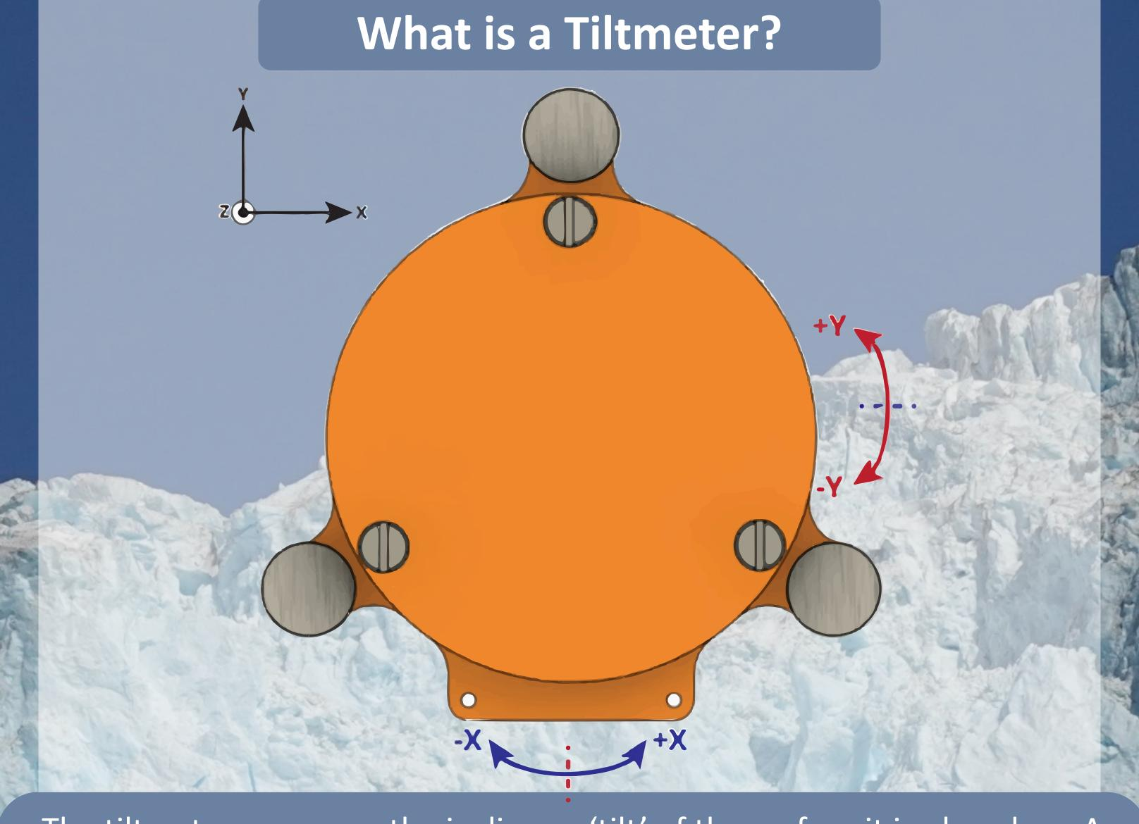
The tiltmeter measures the incline or 'tilt' of the surface it is placed on. A positive Y indicates that the front of the tiltmeter has dipped down with a negative Y showing that the back had dipped down. A Positive X indicates the right side of the tiltmeter had dipped and a negative X would be a dip of the left side.
