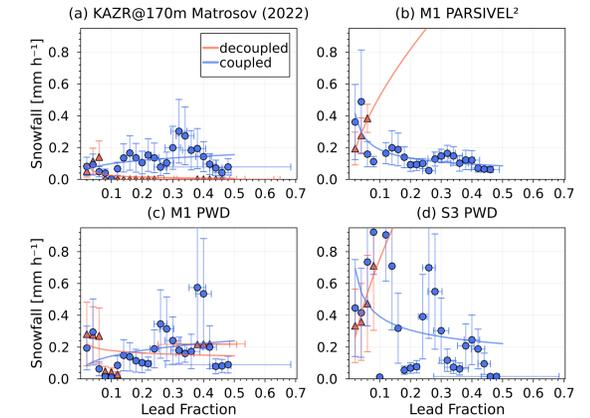
Figure 8: Snowfall rate as a function of Lead Fraction for coupled and decoupled cases: (a) KAZR as [3], (b) PARSIVEL<sup>2</sup>, (c) Present Weather Detector (PWD) on RV Polarstern (M1), (d) PWD on ice floe (S3).
