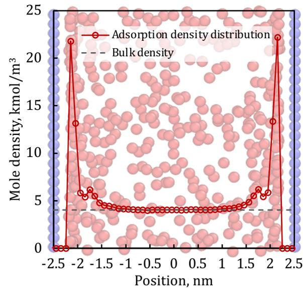
Density profiles of CH<sub>4</sub> in a 5nm pore connected to a non-confined pore at 10MPa and 333K
