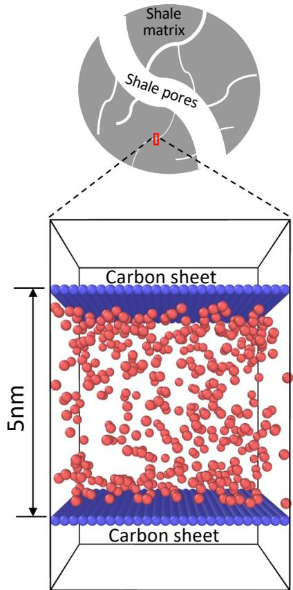
Molecule distributions of CH<sub>4</sub> in a 5nm pore connected to a non-confined pore at 10MPa and 333K
