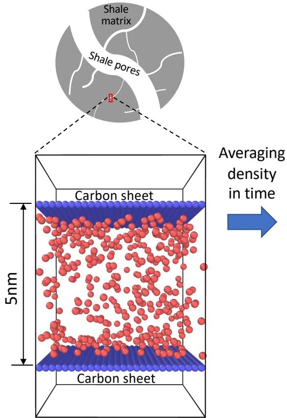
Molecule distributions of  $\text{CH}_4$  in a 5nm pore connected to a non-confined pore at 10MPa and 333K
