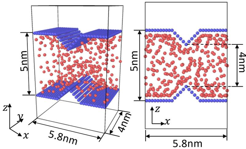
□ Nanopores with rectangle structure on surface
