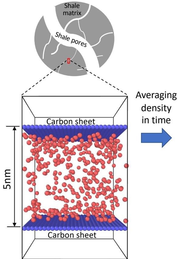
Molecule distributions of CH<sub>4</sub> in a 5nm pore connected to a non-confined pore at 10MPa and 333K
