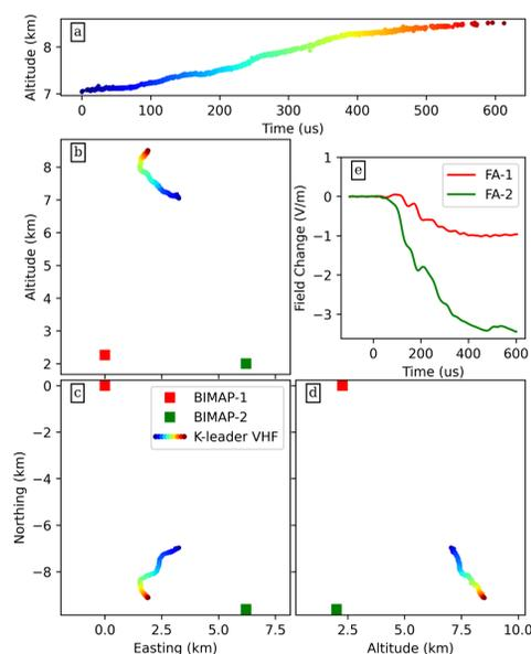
**Figure 1.** Plot of BIMAP-3D data for one dart leader, showing altitude vs time (a), altitude vs easting (b), northing vs easting (c) and northing vs altitude (d), including the location of the two BIMAP stations. The dart leader sources are colored by time. We also include the field change vs time (e).
