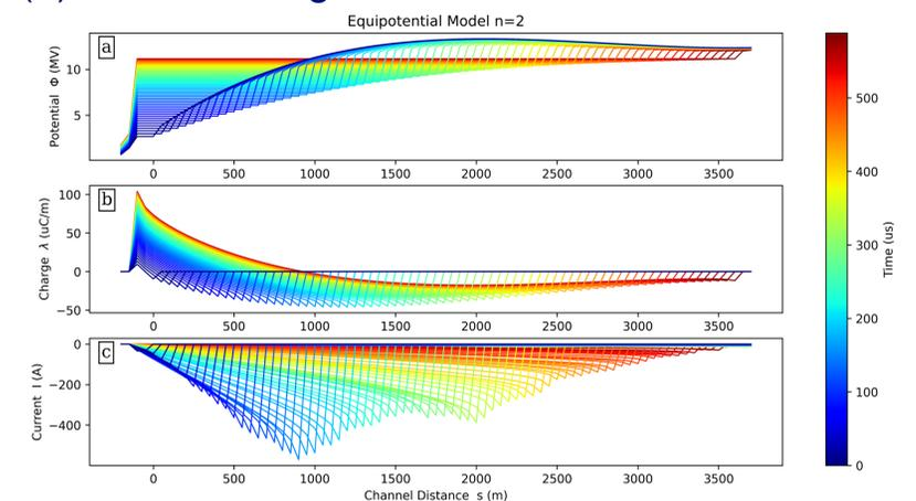
**Figure 4.** Plots showing the potential (a), linear charge density (b), and current (c), all plotted against distance along the channel. Each curve shows a snapshot of the channel at a time indicated by the color.
