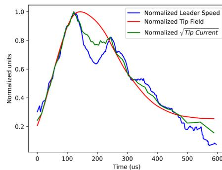
**Figure 3.** A plot comparing the measured leader speed, modeled tip field, and square root of the modeled current, all plotted against time. Each variable on the y-axis is normalized so that its maximum value is 1.
