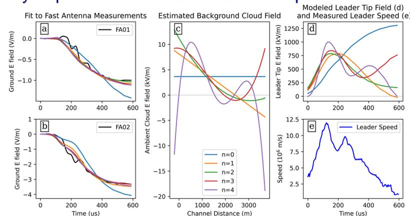
**Figure 2.** Comparison of the measured and modeled ground electric field vs time for FA01 (a) and FA02 (b), the estimated ambient cloud field vs distance along the channel (c), and the modeled tip field vs time (d). The measured leader speed vs time (e) is included for comparison.
