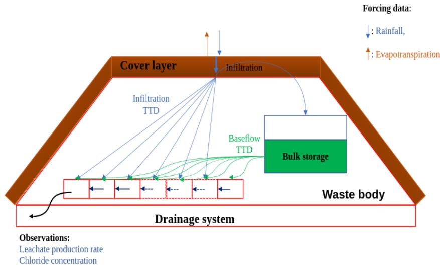
**Figure 1.** A schematic overview of model structure.
