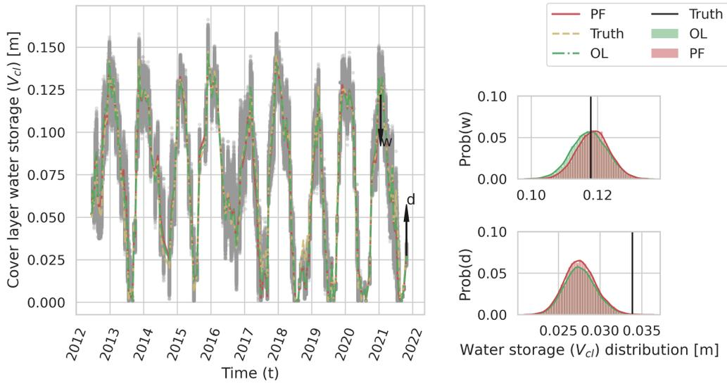
**Figure 2.** Water storage in the cover layer (scenario A). The red line represents the mean estimation of the particle filter. The green and yellow lines represent the open loop results and synthetic truth, respectively. The individual particles are shown as grey points. The two black arrows point to the wet and dry period during the assimilation process, with corresponding probabilities plotted. The black vertical lines in the probability histograms are the truth at specific time steps.
