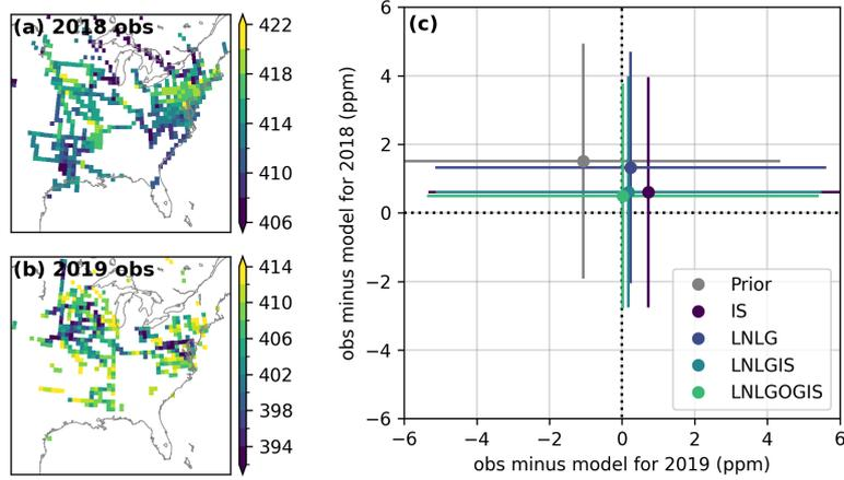
**Figure S12.** Median plus/minus standard deviation of the obs minus model difference for  $\Delta$ NEE-sensitive atmospheric CO<sub>2</sub> measurements in 2018 versus 2019 (see Text S1). These statistics are calculated across all individual observations that qualify as flood-sensitive.
