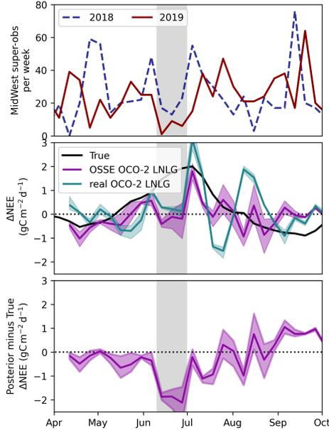
**Figure 4.** Weekly timeseries of (top) number of OCO-2 super-obs in the US Midwest for 2018 and 2019. (middle) Weekly  $\Delta\text{NEE}$  in the US Midwest for the truth, OCO-2 OSSE and real OCO-2 LNLG experiment. (bottom) Difference between posterior and true  $\Delta\text{NEE}$  for the OCO-2 OSSE. The shading shows the range around the mean estimate for the inversions using three different priors.
