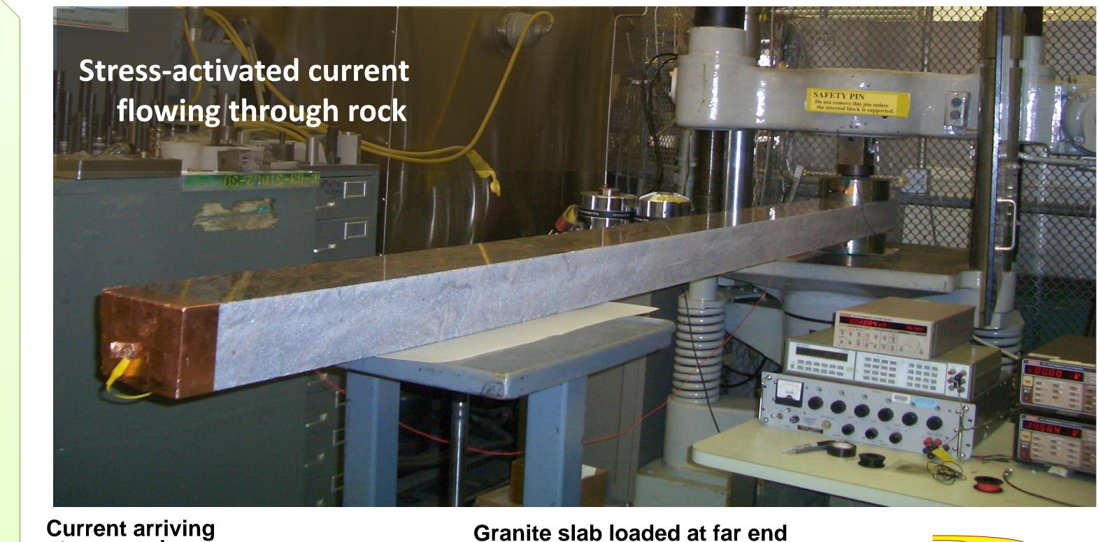
Current arriving at near end Granite slab loaded at far end h\* \_\_\_\_\_\_h\* \_\_\_\_\_
