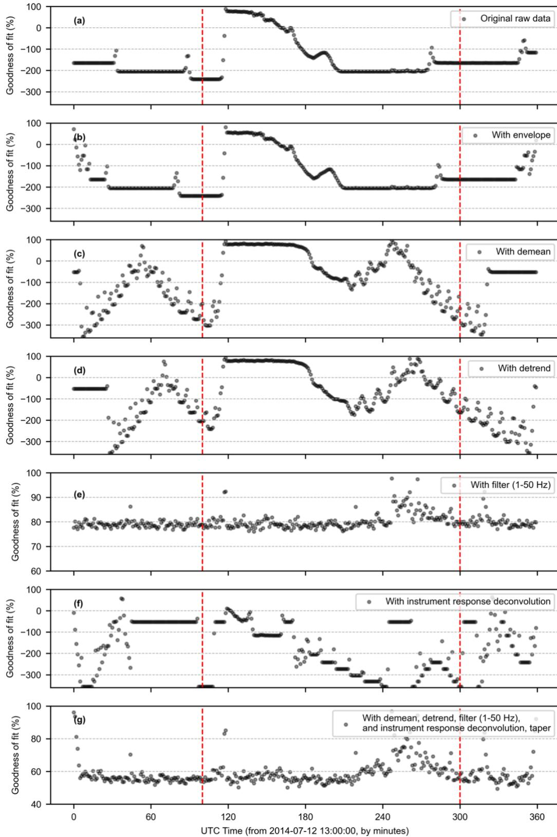
**Figure S1.** Effects of data processing methods on BL, coding by R ESEIS [Dietze \(2018\)](#). The red dashed vertical lines are manually labeled start and end time. The codes are available in **4. Codes**.
