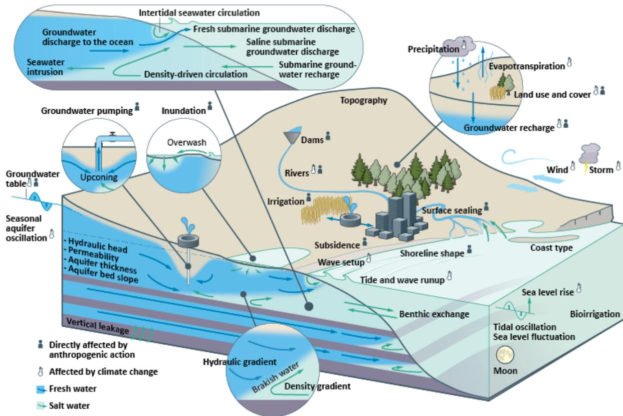
172 **Figure 1.** A perceptual model of coastal groundwater fluxes showing drivers of SGD and SWI,
