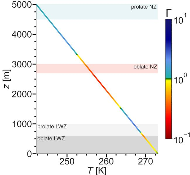
**Figure 15.** Background atmosphere for the 1-D model simulations incl. the vertical profiles of temperature and corresponding IGF. The nucleation (NZ) and liquid water zones (LWZ) are situated in the shaded regions for the respective cases.
