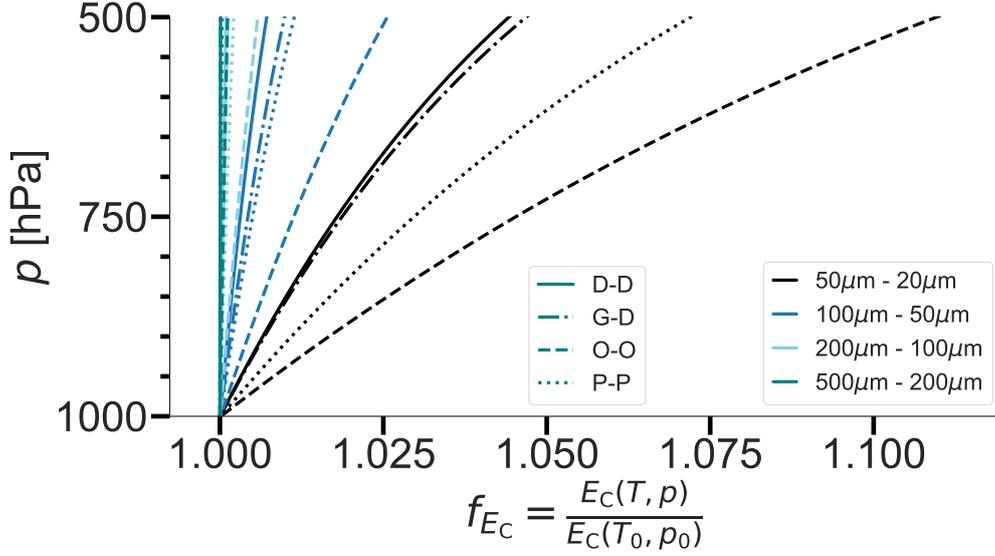
**Figure 6.**  $p$ -profiles of  $f_{Ec}$  for a drop-drop (D-D, solid), graupel-droplet (G-D, dash-dotted lines), an oblate-oblate (O-O, dashed), and a prolate-prolate collision (P-P, dotted). Color-coded is the equivalent diameter of the colliding particles.
