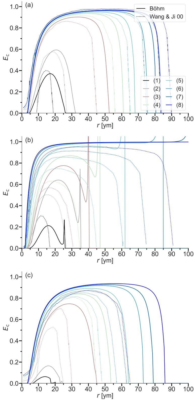
**Figure 8.** Collision efficiencies of a) thin oblates, b) cylinders, and c) broadly branched crystals with spheres. Particle dimensions and reference numerical simulations of Wang and Ji (2000).
