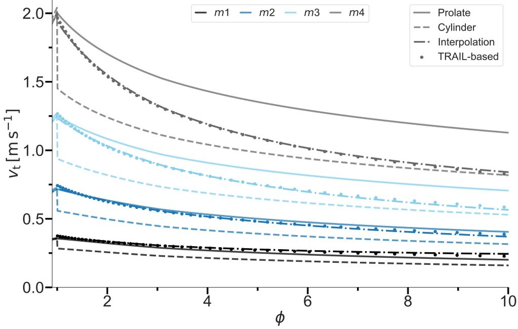
**Figure 3.** Terminal fall speed  $v_t$  dependency on the aspect ratio  $\phi$  for particles with different mass (color-coded), treated as a prolate (solid) or a cylindrical spheroid (dashed), for TRAIL-based data (points), and for an interpolated approach (dash-dotted line, Eq. 31).
