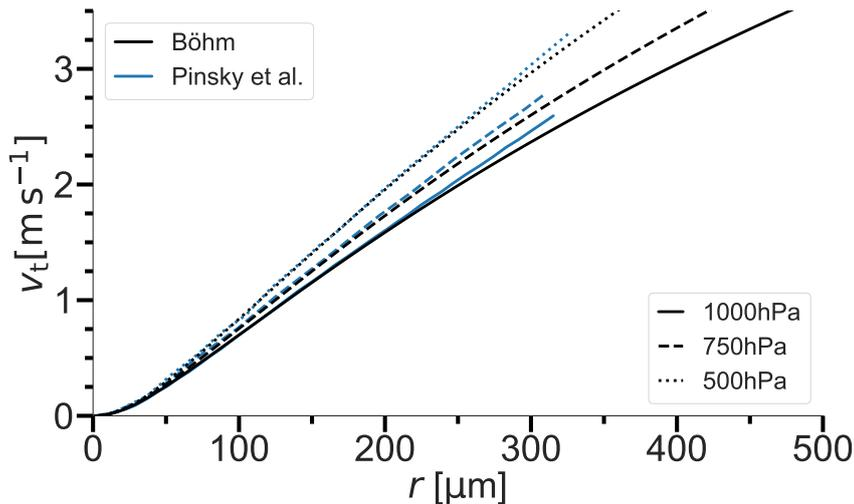
**Figure 4.** Dependency of  $v_t$  on the drop radius for the pressure levels 1000 hPa (solid), 750 hPa (long dashed), 500 hPa (short dashed) for Böhm’s scheme (black) and from Pinsky et al. (2001) (blue lines).
