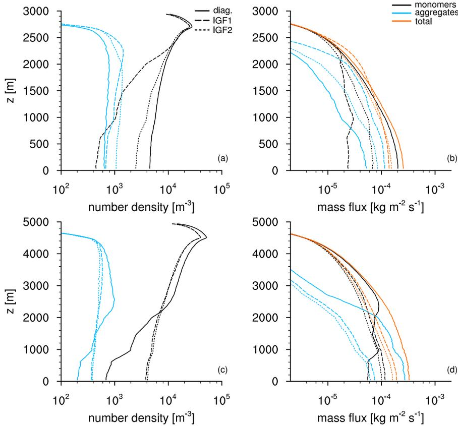
**Figure 21.** Vertical profiles of number density (a & c) and mass flux (b & d) for monomers (black) and aggregates (blue) for the oblate (top row) and prolate (bottom row) nucleation regimes using a diagnostic geometry (solid), HP with original IGF (dashed), and HP with updated IGF (short-dashed) with deposition and aggregation enabled.
