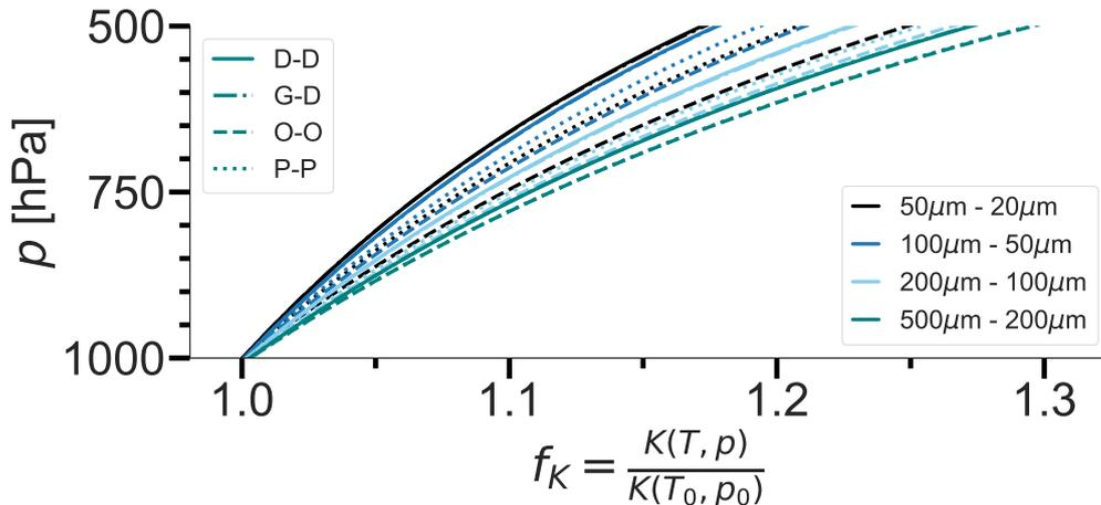
**Figure 7.**  $p$ -profiles of  $f_K$  for a drop-drop (D-D, solid), graupel-droplet (G-D, dash-dotted lines), an oblate-oblate (O-O, dashed), and a prolate-prolate collision (P-P, dotted). Color-coded is the equivalent diameter of the colliding particles.
