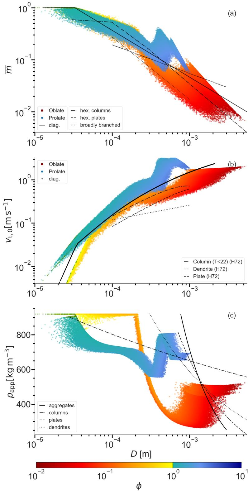
**Figure 16.**  $\bar{m}$ - $D$  (a),  $v_{t,0}$ - $D$  (b), and  $\rho_{app}$ - $D$ -relations (c) for the steady state of the simulation. Markers represent the simulations using a diagnostic geometry and an explicit habit prediction. The particles AR  $\phi$  is color-coded. Lines in (a) are empirical relations of Mitchell (1996), in (b) of A. Heymsfield (1972), and in (c) from Pruppacher and Klett (1997).
