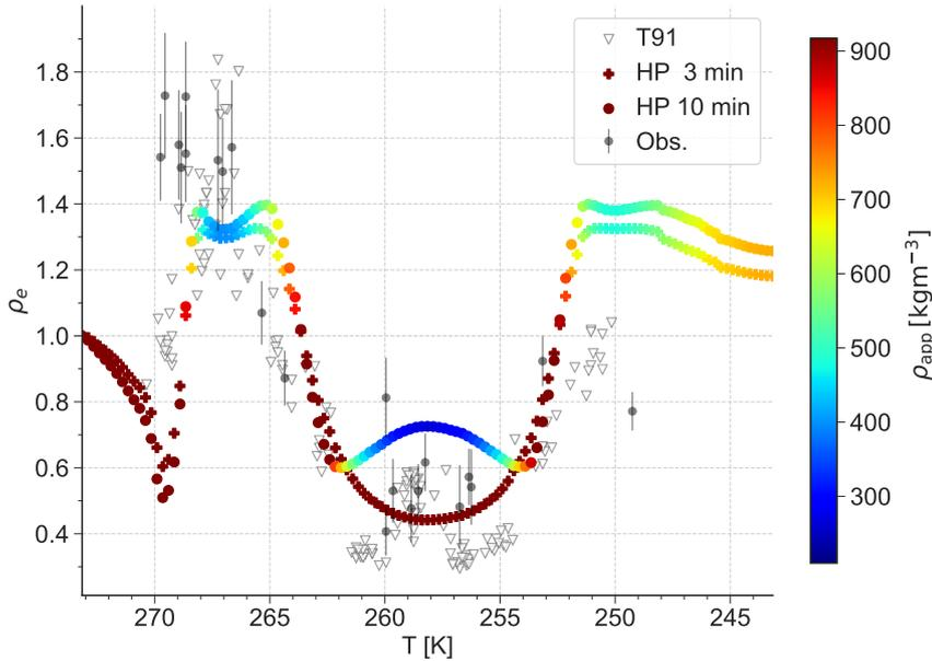
**Figure 11.**  $T$ -dependence of polarizability ratios  $\rho_e$  for ice crystals grown in the free-fall chamber (open grey triangles), with HP ([+] for  $t = 3$  min, [•] for  $t = 10$  min), and observed near cloud tops (black squares, error bars represent  $\pm 1$  standard deviation). Color-coded is the particle's apparent density  $\rho_{\text{app}}$ .
