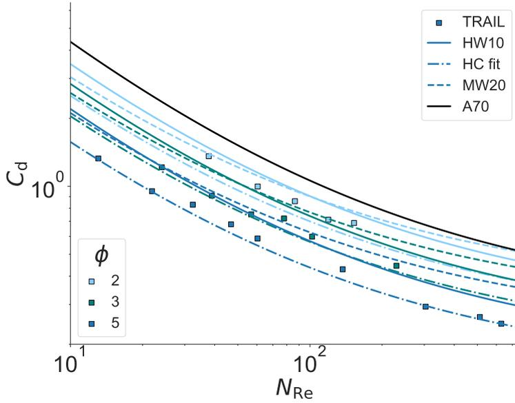
**Figure A1.** Fits for the  $N_{Re}$ - $C_d$ -relations compared with data of hexagonal columns from TRAIL (colored squares). Black line corresponds to the solution of spheres by Abraham (1970, A70), solid lines are the generalized relation of A. J. Heymsfield and Westbrook (2010, HW10), dashed lines mark results of McCorquodale and Westbrook (2021, MW20), and dash-dotted lines show our fit for hexagonal columns (HC) only. The assumed aspect ratio is color coded
