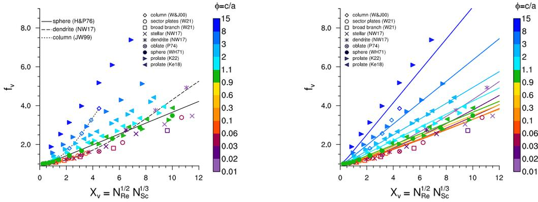
**Figure 9.** Left: Data points and functional dependencies of  $f_v(X_v)$  for several studies. Right: Proposed functional habit-dependent description  $f_v(\phi)$ . The aspect ratio of the assumed particles is color-coded.
