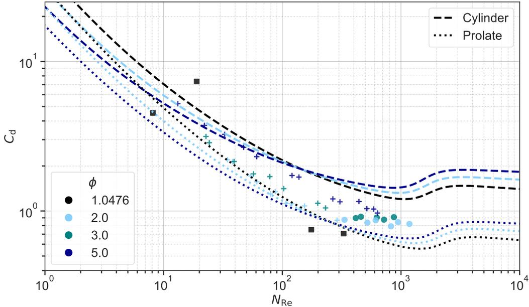
**Figure 2.** Comparison of  $N_{Re}$  and  $C_d$  for measured prolate ice particle analogues from McCorquodale and Westbrook (2021) ('+'/'o' for steady/unsteady regimes) and Westbrook and Sephton (2017) (squares) against the parameterization of Böhm for different  $\phi$  (color-coded) and assumed hydrodynamic assumption (short-dashed: prolate, long-dashed: cylinder).
