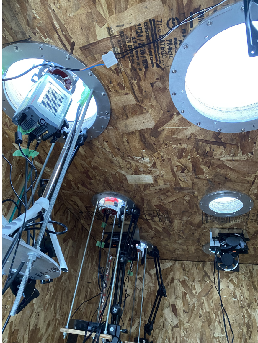
Figure 3. Image from the bottom of the LAMP mission Venetie camera observatory. The skylights are dome shaped to allow the camera lenses to view the entire sky. In the image, cameras are installed in three domes, and three are empty.
