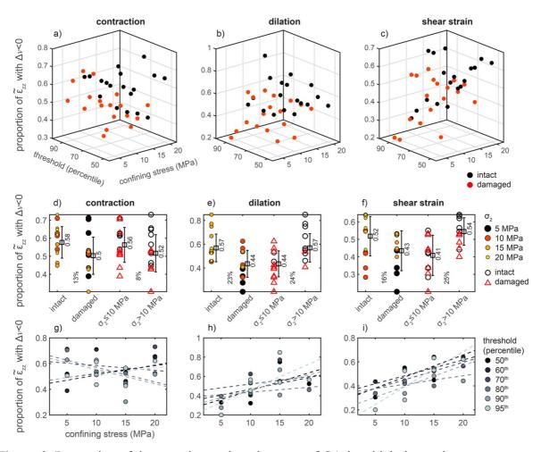
Figure 9. Proportion of the experiment time, in terms of  $\widetilde{\varepsilon}_{zz}$ , in which the strain component produces negative  $\Delta v$ , and thus localizes. Format is the same as Figure 6. The intact rocks experience larger proportions of  $\widetilde{\varepsilon}_{zz}$  in which the strain components localize than the damaged rocks. The experiments with larger confining stress generally host more  $\widetilde{\varepsilon}_{zz}$  in which the strain components localize.
