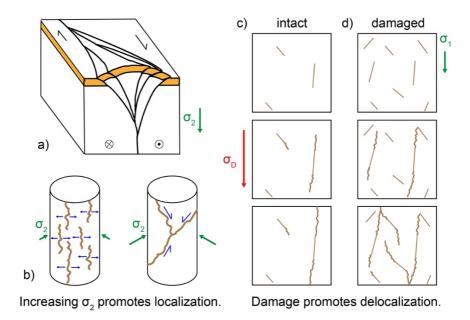
**Figure 12.** Examples of increasing confining stress promoting localization (a-b), and preexisting damage promoting delocalization (c-d). a) Positive flower structures that develop along strike-slip fault networks host a diffuse network of fractures at the surface that localize
