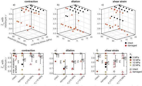
**Figure 10**. Timing of the maximum localization, minimum v, in terms of  $\widetilde{\varepsilon_{zz}}$ . Format is the same as **Figure 6** (a-f). The intact rocks tend to host their maximum localization immediately preceding failure, when  $\widetilde{\varepsilon_{zz}}$  is one. In contrast, the damaged rocks host their maximum localization earlier in loading.
