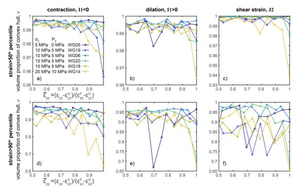
**Figure 5**. Evolution of the volume fraction of the convex hull around the high strain values, v, for strains greater than the 50<sup>th</sup> percentile (a-c) and 90<sup>th</sup> percentile (d-f), for the absolute
