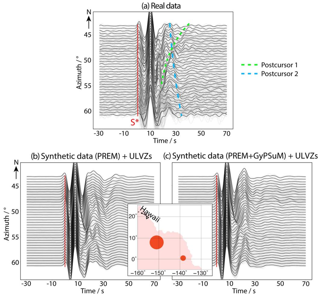
**Figure 5.** Real (a) and synthetic (b,c) transverse velocity seismograms for event 1, including both ULVZs (see inset). Plotting conventions for each subfigure are the same as in Figure 2a. Postcursors are only marked by dashed lines in panel a. (b) Synthetic seismograms for isotropic PREM as background model. (c) Same as (b) for PREM+GyPSuM. Inset: Geographical locations of modeled ULVZs (red circles). Pink colors mark the extent of the Pacific LLVP.
