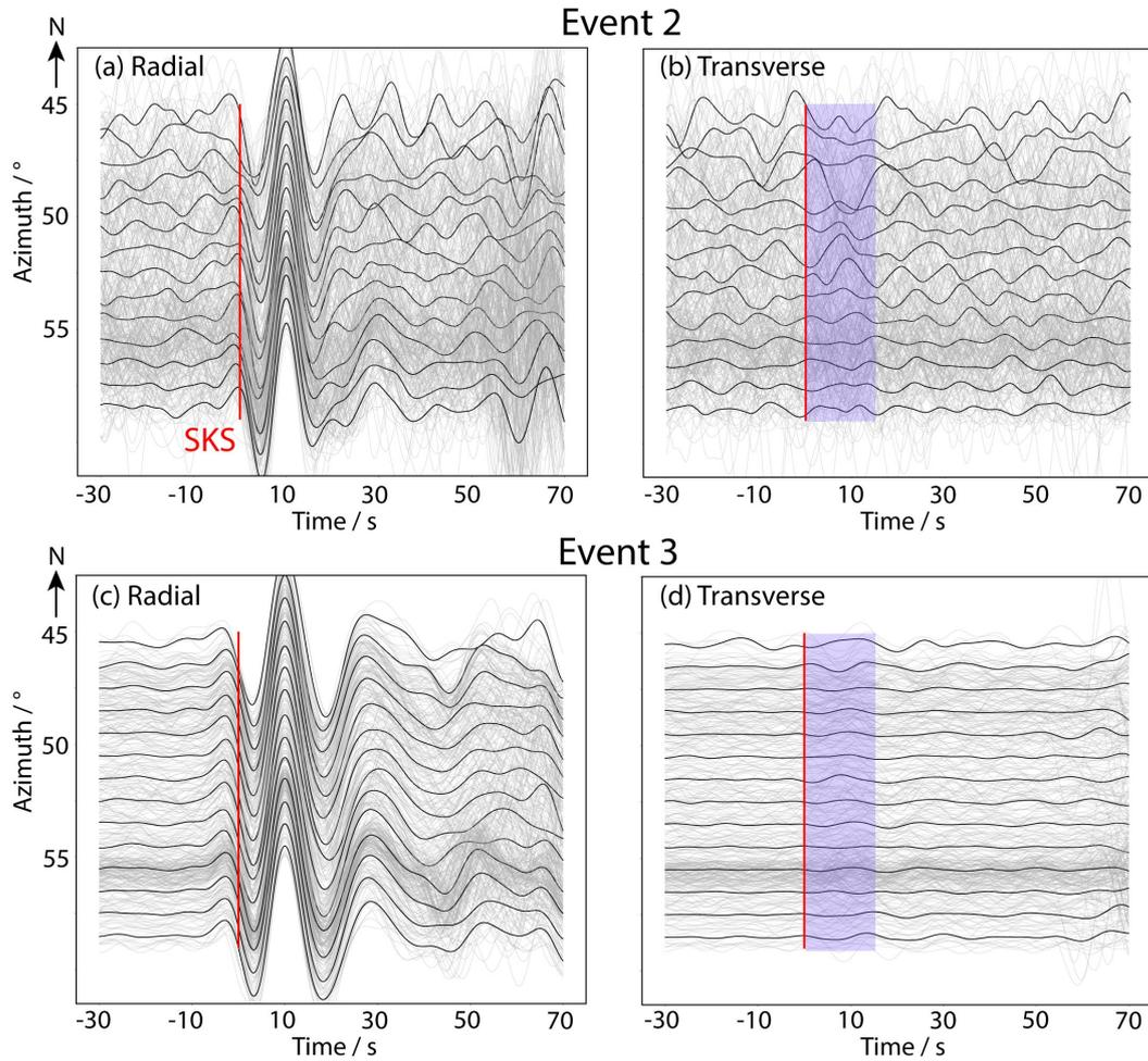
**Figure 6.** Radial (a,c) and transverse (b,d) SKS velocity seismograms as a function of azimuth for events 2 (a,b) and 3 (c,d). Plotting conventions for each panel are similar to Figure 2a. Red solid lines indicate the approximate SKS arrival times, and blue shading marks arriving SKS transverse component energy. For events 2 and 3, an average of 28 traces contribute to each azimuth bin.
