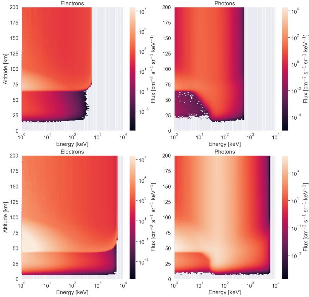
**Figure 5.** Altitude-energy histogram plots of number flux from (top row) a 500 keV and (bottom row) 5 MeV electron beam at an isotropic pitch angle distribution, showing (left column) electron flux and (right column) photon flux. The input flux for both energies is  $10^4 \text{ cm}^{-2} \text{ s}^{-1} \text{ sr}^{-1} \text{ keV}^{-1}$ .
