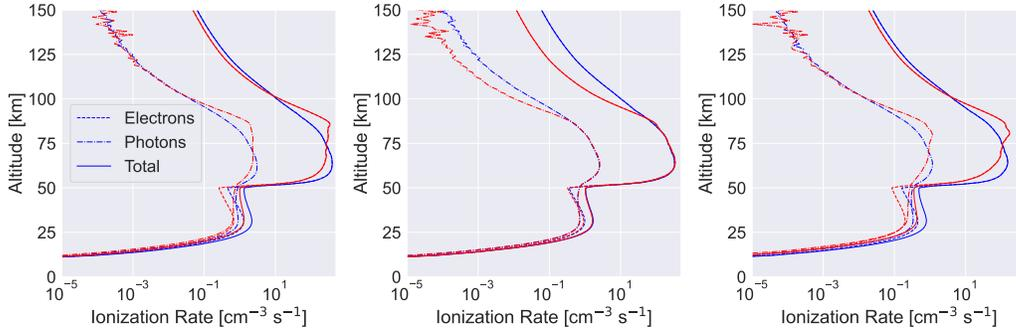
**Figure 16.** Predicted atmospheric ionization response from ELFIN data, performed with the methods described in Section 6.3: method 1 (blue) fits a surface to backscattered electron data and inverts to ionization profile, and method 2 (red) directly forward models loss cone data.
