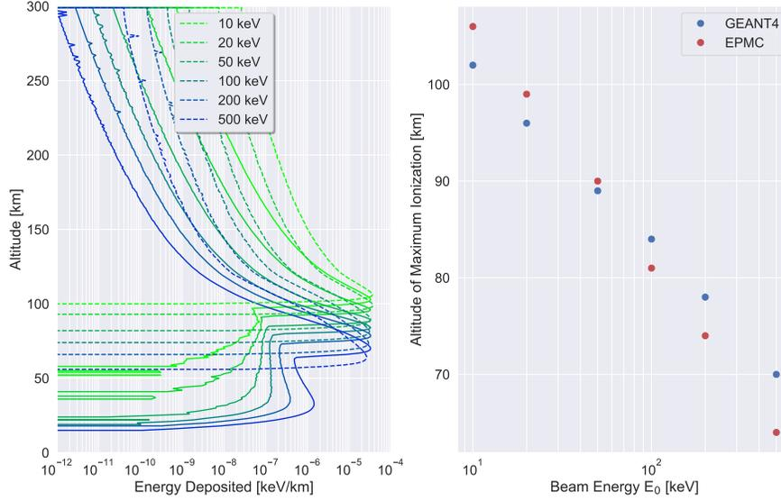
**Figure 11.** (Left) GEANT4 (solid lines) and EPMC (dashed lines) normalized energy deposition profiles with an isotropic pitch angle distribution at 6 energies up to 500 keV. (Right) Altitude of the maximum ionization peak with electron beam energy.
