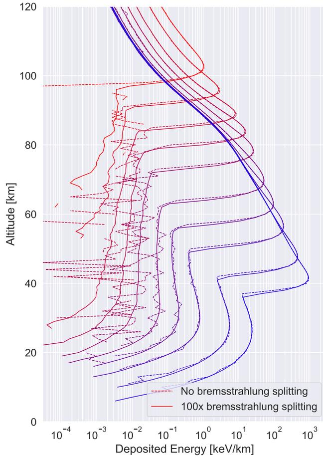
**Figure 2.** Profiles produced by simulating  $10^5$  electrons at energies of 10, 20, 50, 100, 200, and 500 keV (red to blue). Each profile is run with a 100x numerical bias towards bremsstrahlung enabled. A comparison with and without the biasing method is shown here using an isotropic pitch angle distribution.
