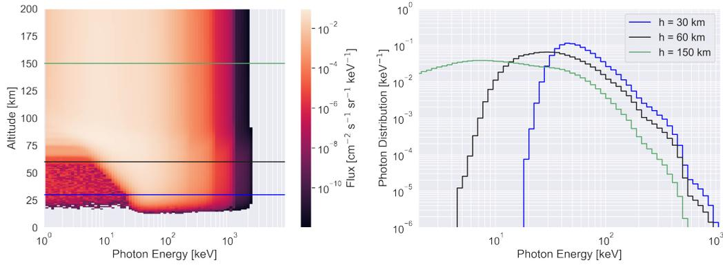
**Figure 10.** (Left) Photon altitudinal spectra for a precipitation event with differential flux  $10^5 \text{ cm}^{-2} \text{ s}^{-1} \text{ sr}^{-1} \text{ keV}^{-1}$  and exponential energy distribution with folding energy  $E_0 = 100 \text{ keV}$ . Note the low flux bins in the lower left-hand corner are from noise. (Right) Altitude-integrated X-ray spectra averaged at altitudes 30, 60, and 150 km, averaged over a  $\pm 5 \text{ km}$  altitude bin.
