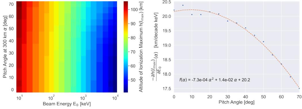
**Figure 4.** (Left) Altitudes of maximum ionization with beam energy and pitch angle. (Right) The rate of change of altitude of peak ionization with beam energy with varying pitch angle. A 2<sup>nd</sup> order polynomial fit is included to show the trend in  $\partial h/\partial E_0$  with pitch angle, where  $\alpha$  is in radians.
