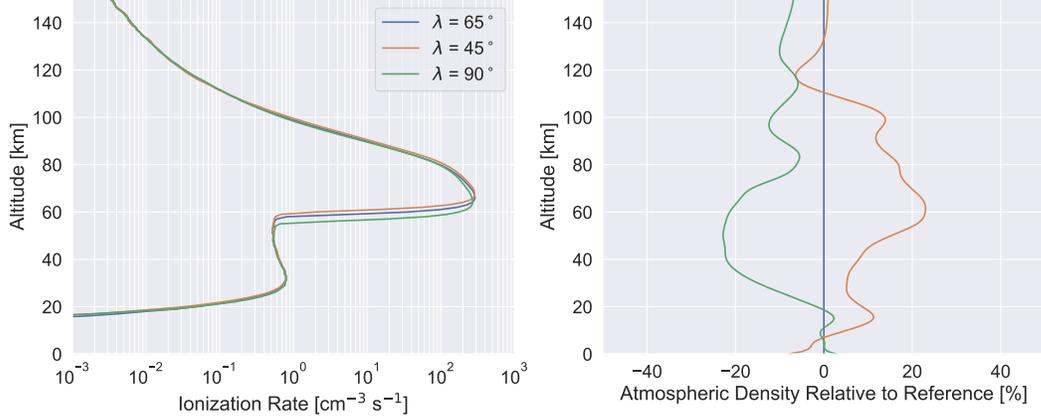
**Figure 9.** Atmospheric ionization rate for the same initial conditions for three atmospheric density profiles and magnetic inclinations. The latitude of PFISR  $65^\circ$  is taken as the reference latitude for atmosphere and inclination angle.
