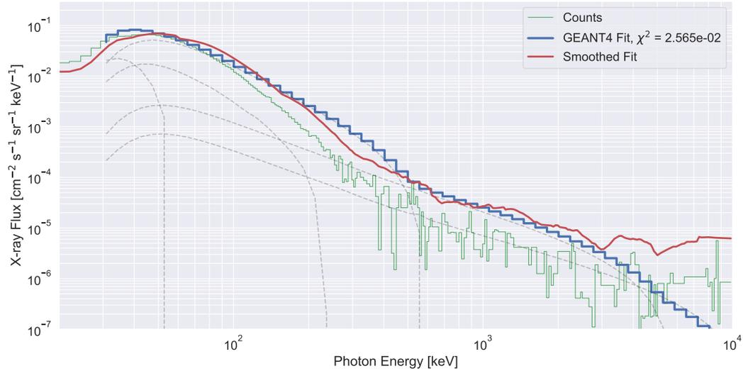
**Figure 13.** BARREL instrument counts per energy bin are shown in green and are adjusted down by the geometric factor to match the order of magnitude of the red line, which are an estimate of physical flux given some an estimate of NaI detection efficiency and is smoothed. The blue stairs plot is the linear combination of Green’s function X-ray spectra (shown component-wise in dashed grey line) that is iterated upon until it matches the BARREL photon flux spectrum.
