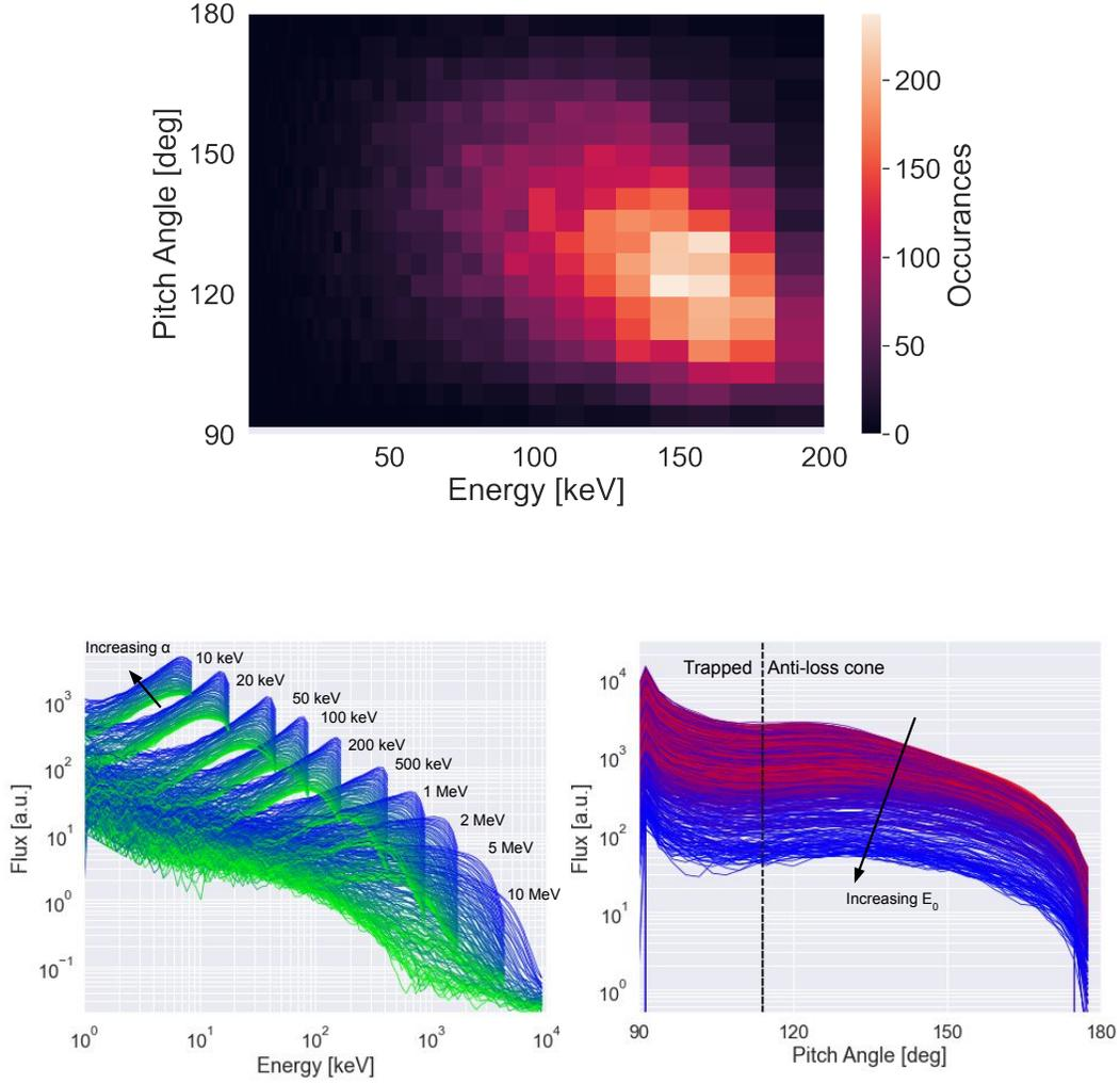
**Figure 6.** (Top) An example of the coupled energy-pitch angle distribution recorded at 500 km that is output from the model. This distribution comes from an input energy of 200 keV and input pitch angle of  $50^\circ$ . (Bottom) One dimensional integrations of the backscattered electron energy-pitch angle spectrum recorded at 500 km altitude for the range of input energies, showing the characteristic rising-energy spectrum for low to medium energies.
