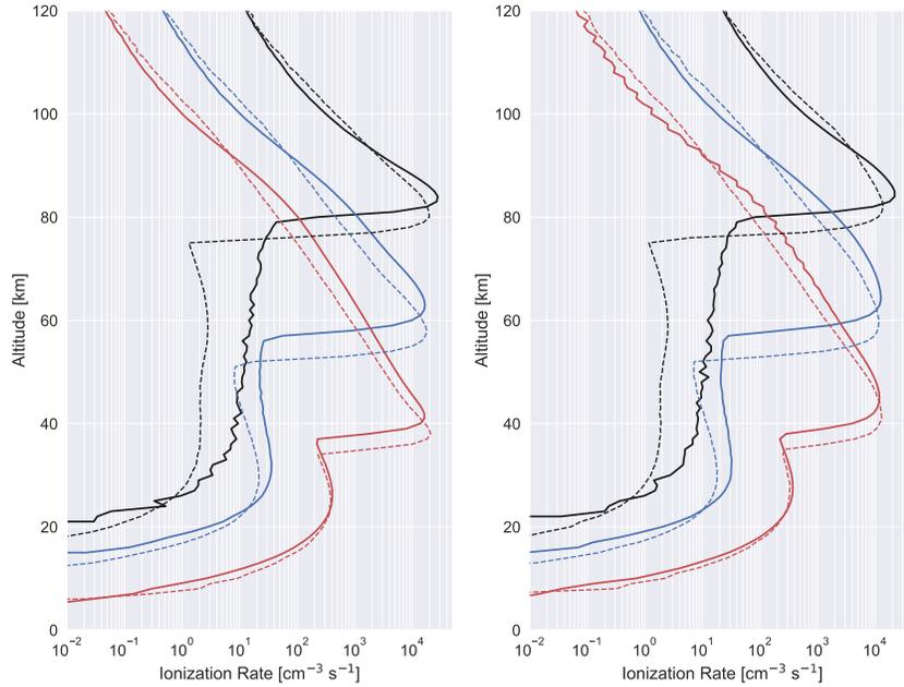
**Figure 12.** Comparison between ionization profiles generated by Xu et al. (2018) (dashed lines) and the GEANT4 model presented in this work (solid lines), both of which include photon tracking to lower altitudes. (Left) Simulation run at  $0^\circ$  pitch angle, and (right)  $45^\circ$  pitch angle for energies 100 keV (black), 1 MeV (blue), and 10 MeV (red).
