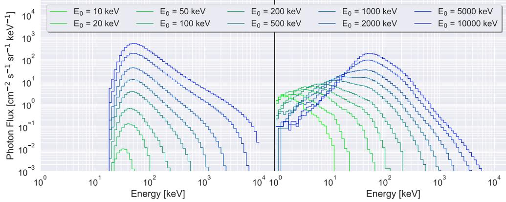
**Figure 8.** X-ray spectra generated from GEANT4 model runs, (left) integrated from 25 – 35 km and (right) 250 – 300 km with isotropic pitch angle and mono energy beams with energy  $E_0$ . The energy of peak flux and slope of the tail increase with increasing  $E_0$ . Note that beam energies of 10 and 20 keV are absent from the left plot since those electron energies do not generate X-rays that reach 25 – 35 km altitude.
