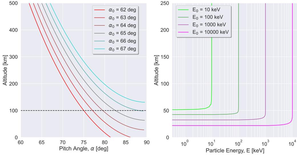
**Figure 1.** (Left) Single particle pitch angle evolution with altitude, where  $\alpha_0$  is the pitch angle at 500 km altitude. The black dashed line marks 100 km, which is the altitude used to define the edge of the loss cone. (Right) Energy evolution with altitude from electrons injected at field-aligned pitch angles. Highlighted here is the relative depth of penetration into the atmosphere with initial particle energy.
