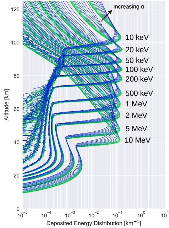
**Figure 3.** Green's function ionization response to mono-energy mono-pitch angle inputs. Variation in pitch angle from field-aligned ( $0^\circ$ , green) to near the edge of the loss cone ( $70^\circ$ , blue) is shown, at pitch angle spacing  $\Delta\alpha = 5^\circ$  and variation in pseudo-log-spaced energies denoted on the plot, with peaks descending in altitude. The deposited energy is normalized to integrate to unity.
