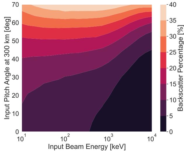
**Figure 7.** Total backscatter from with an input beam energy  $E_0$  and pitch angle  $\alpha_0$  at injection altitude 300 km. At low energies and high pitch angles, only 2/3 of the loss cone population is precipitating in one bounce interaction with the atmosphere.
