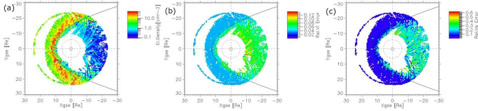
**Figure 5.** MMS fast survey mode data from 2018 as a function of the spacecraft position in the xy GSE plane. (a) shows the electron density measured by FPI. (b) and (c) show the relative error in the bulk velocity for ions and electrons, respectively.
