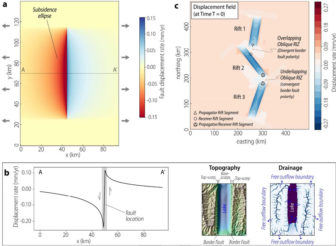
**Figure 5.** Model setup to simulate landscape evolution across two contiguous rift interaction zones with geometries similar to those of the Middle Shire and Nsanje rift interaction zones. **a - b.** Fault segment uplift field with hanging wall subsidence and footwall uplift. Inset maps in panel b shows the resulting topography and drainage for a graben configuration. **c.** Initial displacement field applied in the model to estimate the fault development and rift evolution.
