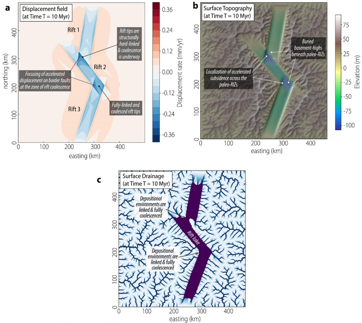
**Figure 8.** a. Displacement field, b. modeled topography, and c. drainage map at 10 Myr showing complete rift coalescence across the tip-to-tip RIZ and established hard-linkage with ongoing coalescence across the overlapping RIZ. Interestingly, the results also highlight that once rift linkage is established, rift coalescence is accompanied by the focusing of accelerated fault displacement and basin subsidence across the deforming RIZs.
