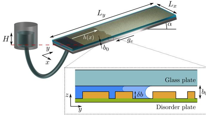
**Figure 1.** Schematic of the model and its experimental realization. Disorder is introduced by randomly placed “mesa defects”—sharp variations in gap thickness,  $b(x, y) = b_0 \pm \delta b(x, y)$ . Imbibition and drainage are driven by raising and lowering the wetting fluid reservoir,  $H$ . The cell is tilted to provide an effective gravity  $g_e = g \sin \alpha$ . The interface configurations  $h(x)$  are recorded by a camera.
