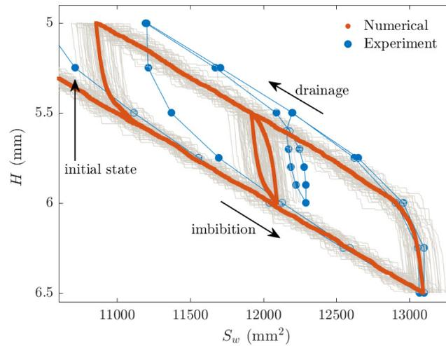
**Figure 4.** Simulated and experimental PS cycles in terms of external head  $H$  and wet area  $S_w$  in the imperfect Hele-Shaw cell shown in Fig. 1, using the same defect statistics. The numerical curve is the result of averaging 52 independent realizations (in gray). The uncertainty of the experimental data (single experiment) is smaller than the symbol size.
