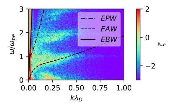
Figure 5: Dispersion relation of the resulting system for  $v_d = 80$ .  $\zeta$  represents the FFT amplitude of the normalized electric field.
