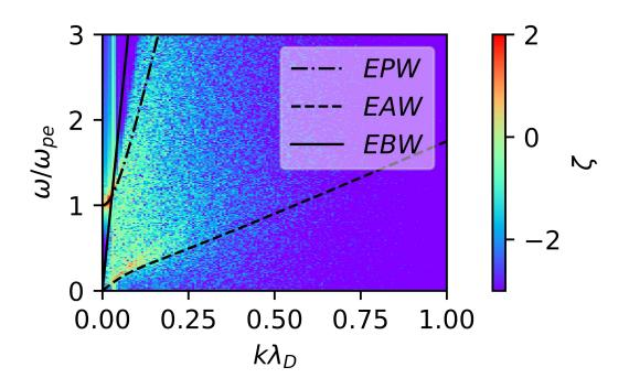
Figure 7: Dispersion relation corresponding to Run-8.  $\zeta$  represents the FFT amplitude of the normalized electric field.
