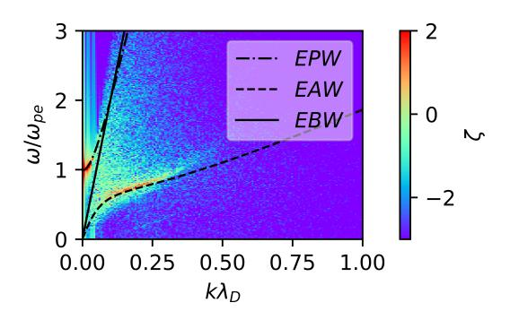
Figure 3: Dispersion relation of the resulting system for  $v_d = 20$ .  $\zeta$  represents the FFT amplitude of the normalized electric field.
