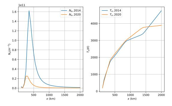
Figure 1: Plot of the electron density and temperature profiles on  $1^{st}$  Feb 2014 and 2020 at Svalbard (77.8750°N, 20.9752°E).
