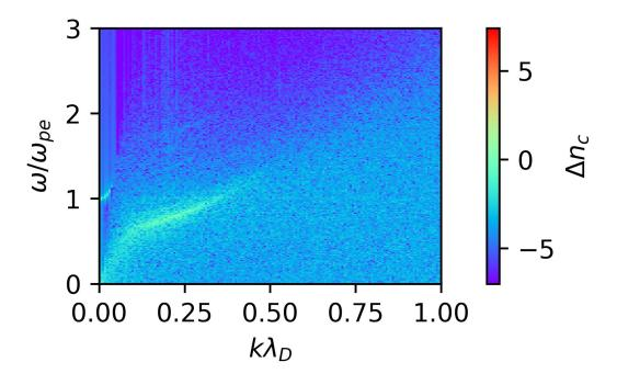
Figure 10: Density fluctuation FFT ( $\Delta n_c$ ) of the cold electrons at  $v_d = 20$ .
