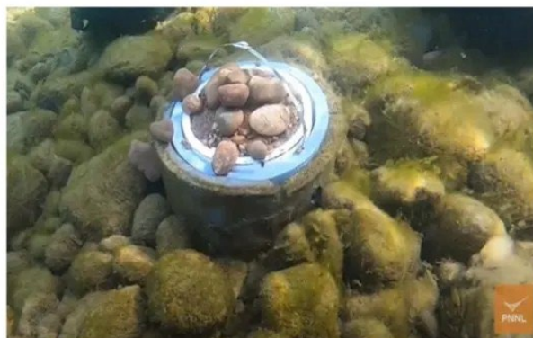
Fig. 4. Photo of POM trap deployed in the Hanford 300 Area riverbed, February 2020. See the following URL for a video of trap deployment and collection: ( https://www.youtube.com/watch?v=jeWB6zTm2o8&fs=1&modestbranding=1&rel=0&showinfo=0 )
