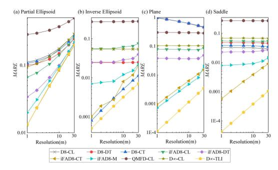
**Figure 5.** The mean absolute relative error (*MARE*) of the estimated flow distance by different algorithms over (a) the partial ellipsoid, (b) the inverse ellipsoid, (c) the plane, and (d) the saddle with six different resolutions. Here the lines of D $\infty$ -TLI and iFAD8-CT are almost coincident for (a) the partial ellipsoid.
