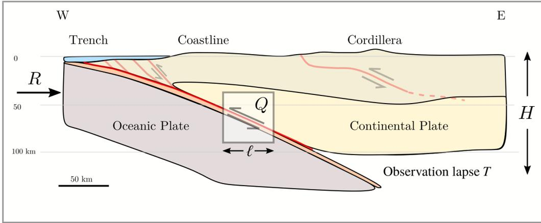
**Figure 1.** Cross section sketch of a subduction border. An energy injection is placed west with a power  $R$ , feeding a complex tectonic process with characteristic geomorphologies (trench, coastline and cordillera) induced by a Continental Plate overriding an Oceanic Plate. Within a volume with proper-length  $\ell$ , a release process  $Q$  takes place across a larger volume with proper-length  $H$ . The observation period  $T$  determines the longer time periods available for study.
