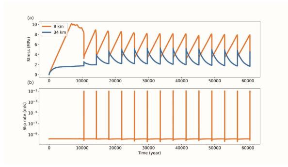
792 Figure 12. Evolution of the stress at the reference point at a depth of 8 km (orange) and 33 km
