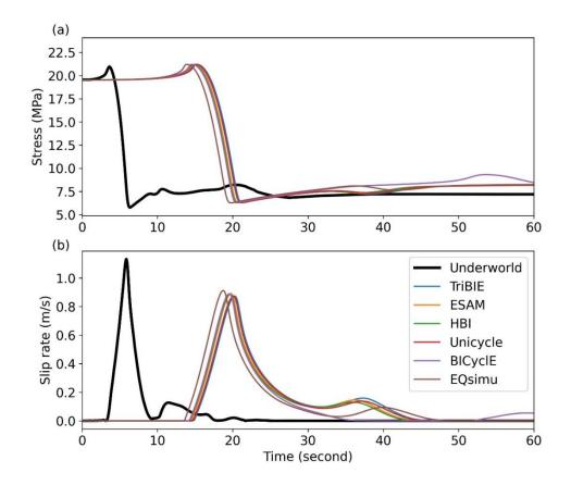
Figure 6. Stress (a) and slip rate (b) at the reference point (0, 0, -10 km) for the first 60 seconds
