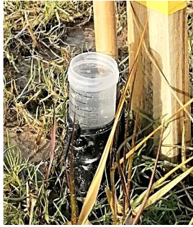
Figure 7. Traps used for the collection of sediment samples over the salt marsh platform.
