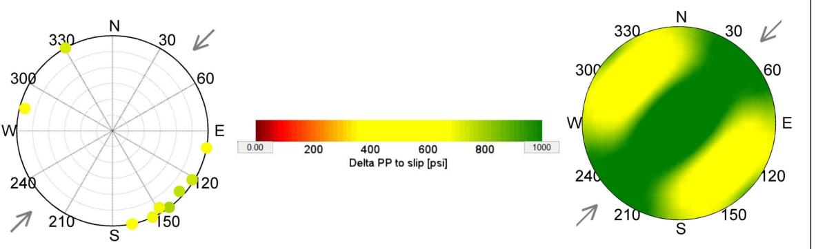
The orientation of the faults as shown in the stereonet diagrams. The arrows represent the direction of maximum horizontal stress.
