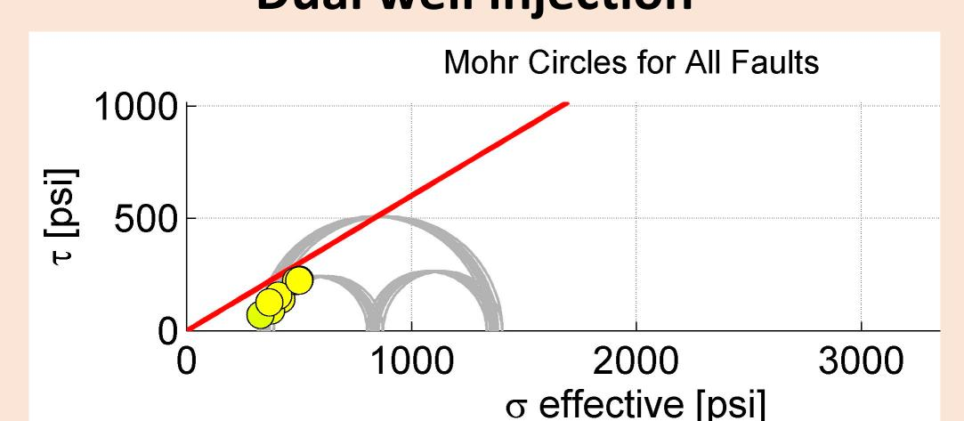
(Deterministic) Risk of fault slip in different injection scenarios represented through Mohr diagrams. Two faults slip in single well injection while no fault slips in dual well injection, even though some faults are close to failure.
