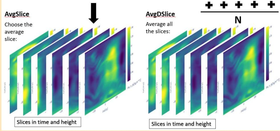
The two **orbit slicing** analysis options are quite similar, only differing in the portions of the orbit used (see medium blue column in table above). Instead of slicing through the model data at specific coordinates, the two analysis methods slice along the satellite trajectory.
