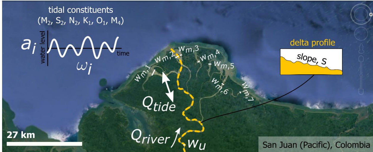
Figure 5. Metrics involved in the calculation of sediment flux by tides, Q_{tide} , from delta morphology, as given for the San Juan River delta (Colombia). In this case, there are seven distributary mouths, with a channel width for each mouth ( w_{m,1} , etc., also applied for fluvial-dominated deltas), measured from the Google Earth® imagery. We calculated the delta slope with an average of elevation change and distance along the transect in yellow. We represent tidal properties by amplitudes and frequencies of tidal constituents. We use Q_{river} to quantify fluvial channel depth (see text for explanation).
