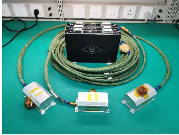
Figure 1. The flight model of the FY-4B FGM includes three sensors and one electronic box.
