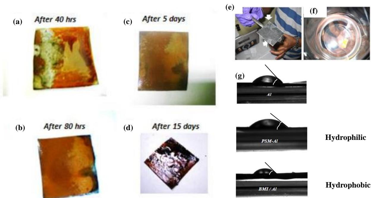
**Fig 3.** The effect of corrosion on mild steel immersed in Ringer's solution for (a) 40 hrs (b) 80 hrs (c) 5 days and (d) 15 days (e) Corrosion on aluminium substrates and (f) no signs of corrosion on BMI coated substrates (g) Contact angle measurements on the surface of Al, PSM-Al, and BMI/Al [5]
