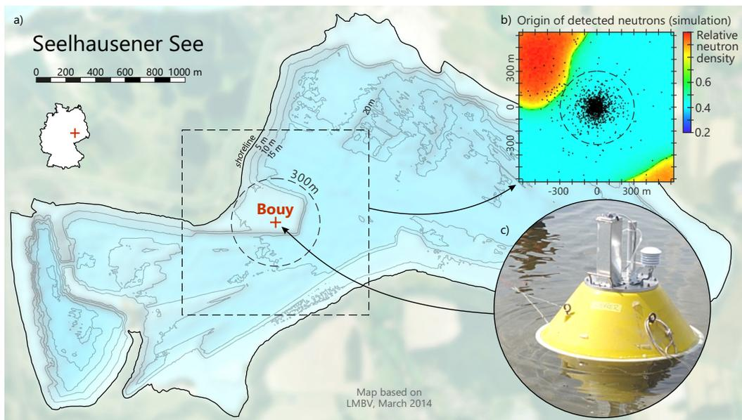
**Figure 1.** a) Location of the CRNS buoy detector at lake *Seelhausener See*. b) The distance of 300 m from the shoreline was chosen such that more than 98,% of detected neutrons had contact to water only (black dots, simulated with URANOS). c) Photograph of the buoy in operation. Map credits: adapted from LMBV, March 2014.
