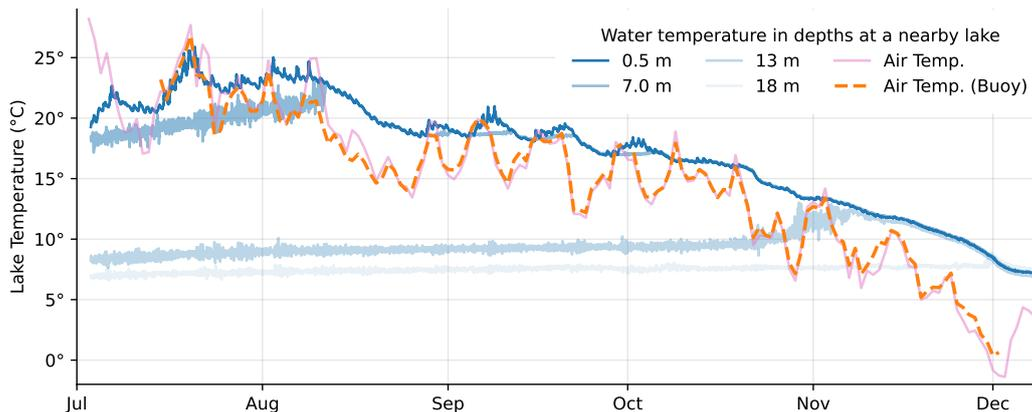
**Figure B1.** Water temperatures measured by an anchored weather station with attached thermistor chain in *Rassnitzer See* from July 2014 to January 2015 in several depths (blue shading). Air temperature has been measured at both lakes, *Rassnitzer See* (pink solid) and *Seelhausener See* (orange dashed).
