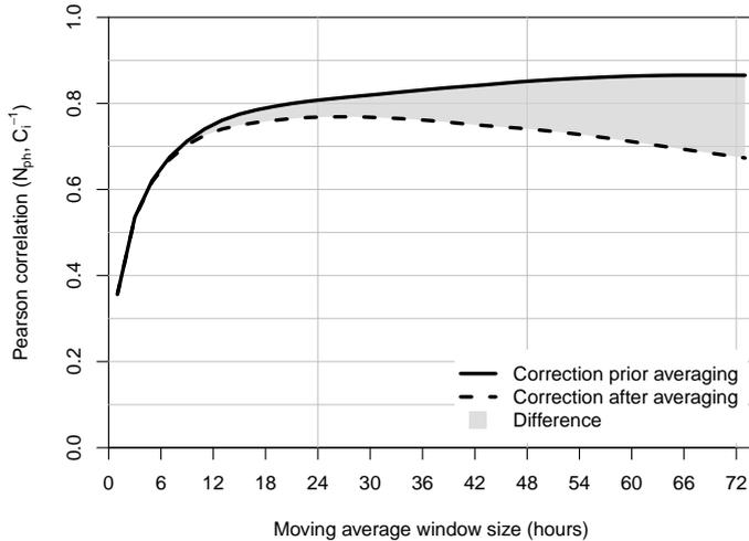
**Figure A1.** Pearson correlation coefficient between the epithermal  $N_{ph}$  vs. inverted influx correction after (Zreda et al., 2012) using the JUNG neutron monitor, when the correction is applied prior or after smoothing with a moving average
