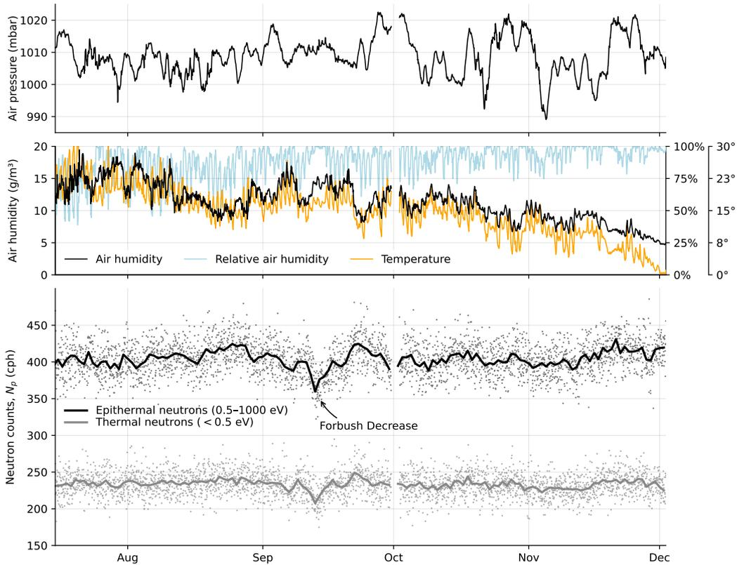
**Figure 3.** Data collected with the buoy instrument in 2014. Top: Air pressure. Middle: External air humidity and temperature. Bottom: pressure-corrected neutron counts of epithermal (0.5–1000 eV, black) and thermal energies (0–0.5 eV, grey). Dots depict hourly measurements, and solid lines depict the daily aggregation. A Forbush decrease event has been detected on September 13th. Maintenance work, including battery exchange, has been conducted on September 30th.
