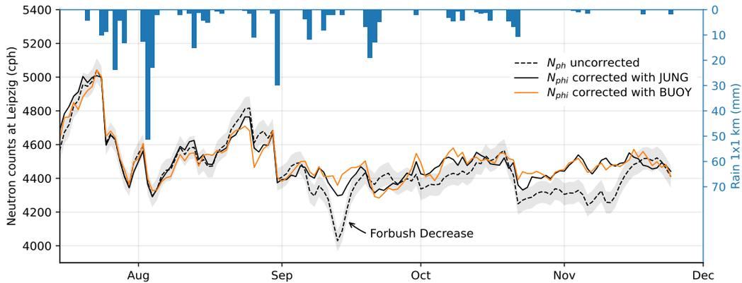
**Figure 7.** Epithermal neutrons aggregated from six collocated CRNS stations at the UFZ Leipzig, 25 km away (Schrön et al., 2018, data from). Neutron counts were corrected for air pressure and air humidity (dashed black) and corrected for incoming radiation using NM Jungfraujoch (solid black) and the buoy data (solid orange). Daily precipitation is indicated from Radolan measurements.
