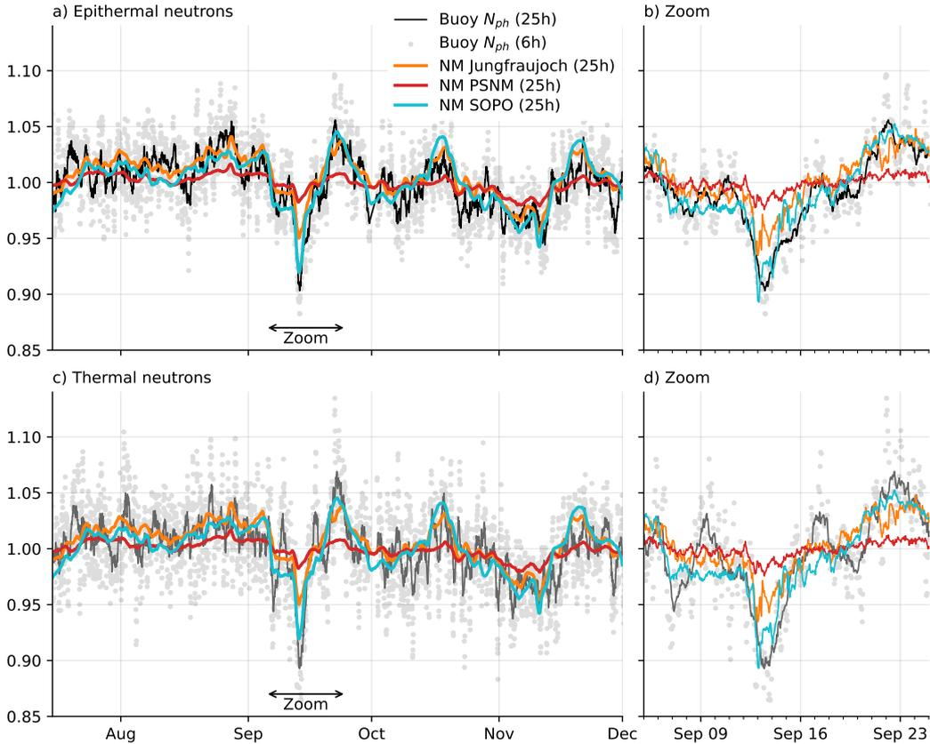
**Figure 6.** Normalized pressure- and humidity-corrected neutron count rates of the buoy detector compared with neutron monitor data. a) Epithermal buoy neutrons with a moving average window of 6 hours (grey dots) and 25 hours (black line). The latter filter was also applied to the NM data from JUNG in Switzerland (orange), PSNM in Thailand (red), and SOPO near the South Pole (blue). b) Zoom-in to the Forbush decrease event. c-d) Same as a-b for thermal buoy neutrons.
