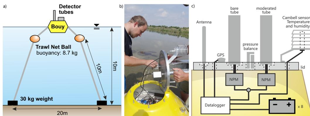
**Figure 2.** a) Setup of the buoy in the lake at around 10 m depth using trawl net balls and weights. b) Final checks with an open lid near the shore before the final launch into the water. c) Detector housing inside the tailor-made lid of the buoy, including GPS, antenna for data transmission, external sensors for air conditions, and a large battery array.
