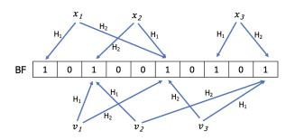
Fig. 3: Elements  $v_1, v_2, v_3$  belonging to the hiding set of Bloom filter of 10 bits storing  $x_1, x_2, x_3$ . Arrows indicate the bits that are set to one according to two hash functions  $H_1$ and  $H_2$ .
