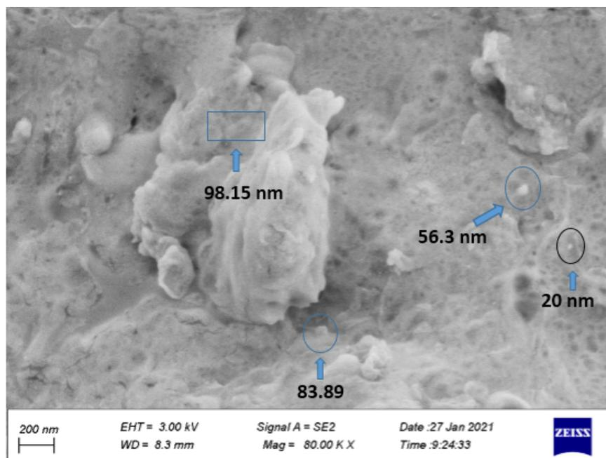
Figure 2: SEM image of CdO nanoparticles and particle size distribution
