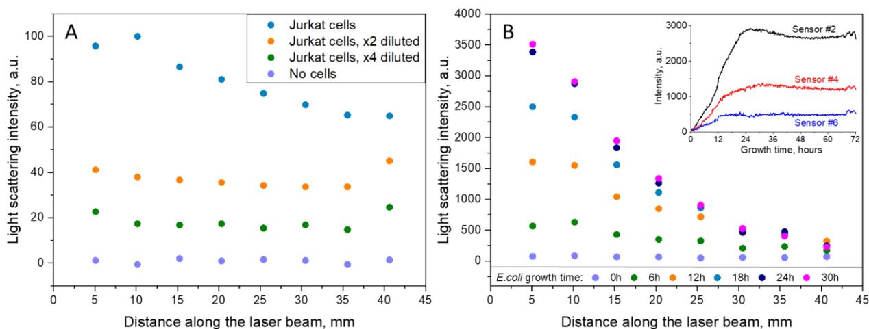
Figure 3. Testing of the prototype with cell cultures. A: Jurkat cells give low but detectable signal, but the attenuation of laser beam is visible only for maximal concentration ( $\sim 10^6$  ml<sup>-1</sup>). B: Continuous monitoring of the *e.coli* bacteria growth.
