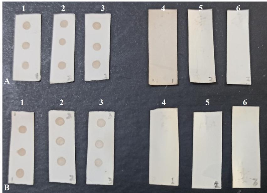
**Fig. 5** Stability of dotted NCM strips after six months of storage at 4 °C and 37 °C. Panel A: Storage of strips at 4 °C; Lane 1-3: GWFI positive serum; Lane 4-6: Goat negative serum. Panel B: Storage of strips at 37 °C; Lane 1-3: GWFI positive serum; Lane 4-6: Goat negative serum.
