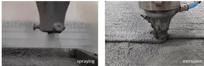
**Figure 3.** Spraying (left) and extrusion (right)
