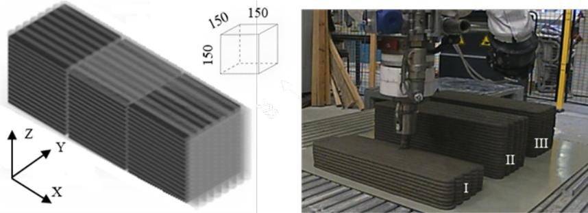
**Figure 1.** Extrusion test specimen: CAD (left) and physical while production (right)
