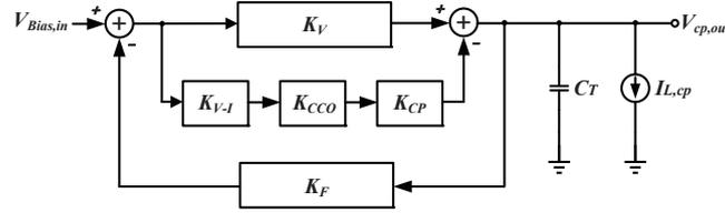
**Figure 4** Simplified model of the proposed closed-loop charge pump.
