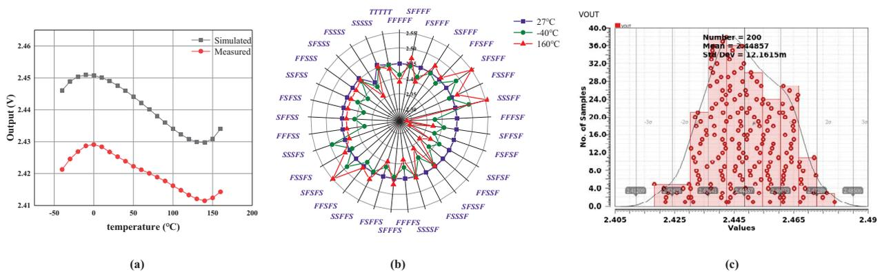
**Figure 10** Simulation performance of output voltage with (a)temperature (b)corner and (c)Monte carlo
