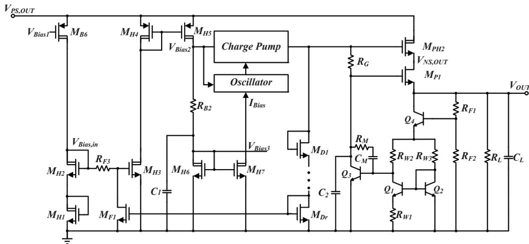
Figure 2 The architecture of the proposed LDO
