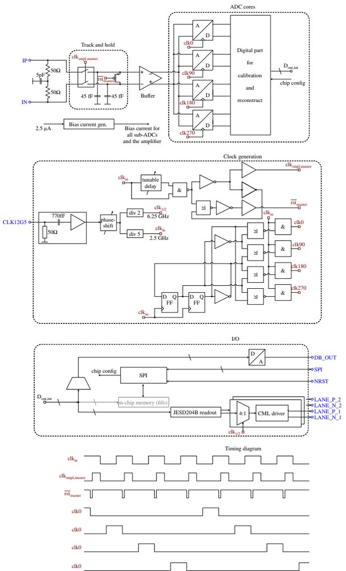
**Fig 1** Block diagram of the entire testchip including I/O and details to clock generation.
