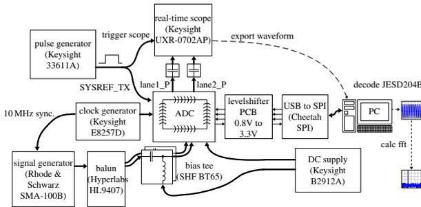
**Fig 2** Block diagram of the measurement setup.
