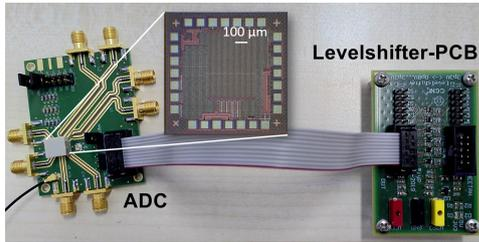
**Fig 3** Microphotograph of chip and PCB used for the measurements.
