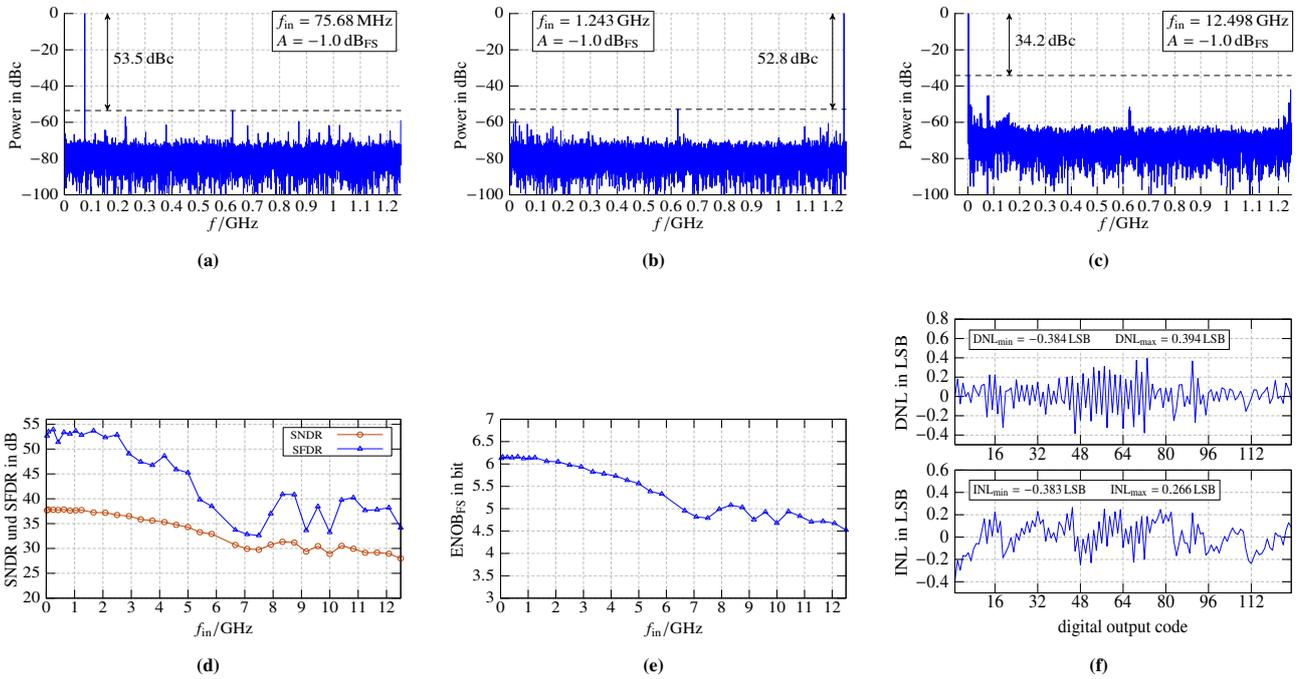
**Fig 4** Measurement results: spectra for different input frequencies and sample rate of 2.5 GS/s (a-c), SFDR, SNDR (d), ENOB (e) against input frequency and static nonlinearities INL, DNL (f).
