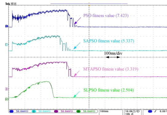
**Fig.7.** The curve of fitness function under condition 1.
