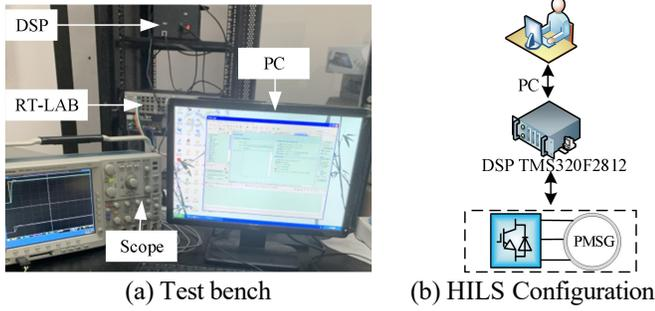
Fig.4 RT-LAB experiment platform
