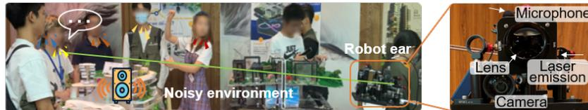
The cocktail party problem, hearing a specific speaker in a loudly noisy environment, is extremely difficult for machines and has become the holy grail in audio processing research. A robotic ear termed REAL (Robot Ear Accomplished by Laser) is devised to accurately recognize human voices in cocktail party environments by remotely probing the vibrations of sound-carrying surfaces by optical means.
