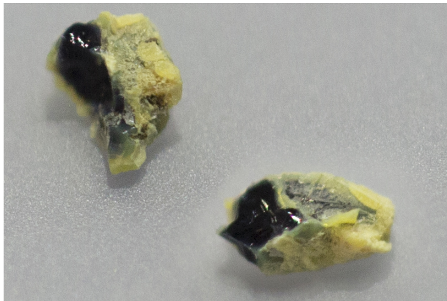
Figure 2. Shrinking core process observed in \text{CH}_3\text{I} adsorption on \text{Ag}^0 -Aerogel, two cut halves of a partially reacted pellet
