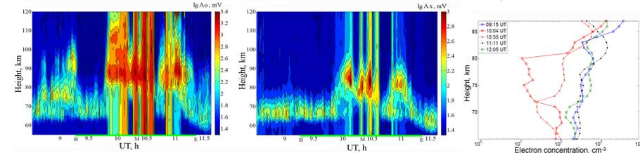
Fig.1. amplitude of ordinary (left) and extraordinary (middle) waves, and electron concentration (right) during the 20 March 2015 eclipse
