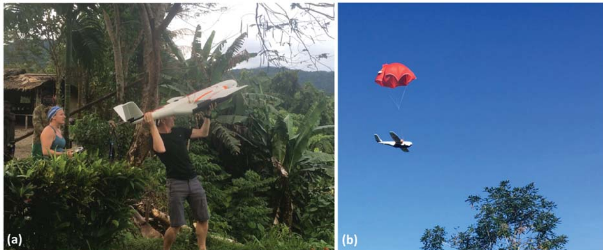
Figure 3. (a) Hand launch of the Titan aircraft, facing into slight wind and from an elevated position on a ridge at 6.159^{\circ} S, 155.137^{\circ} E. (b) Parachute landing of the aircraft in a field adjacent to the take-off site.
